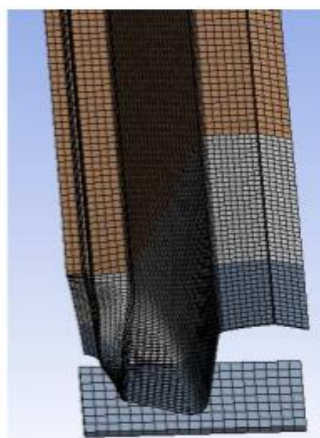
Figure 11 - Symmetric and repetitive web failure mode
