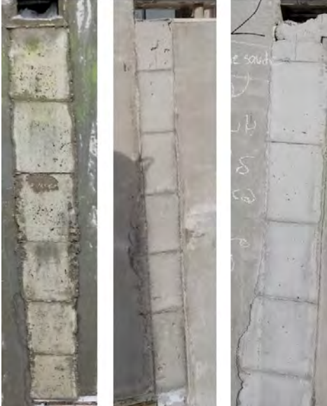
Figure 5-11 Test specimens after grouting (WL1, WL2 and WL3)
