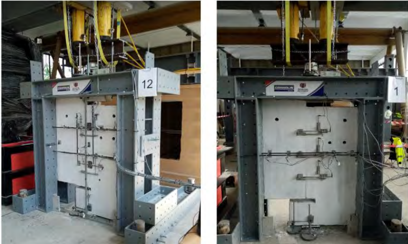
Figure 5-12 Push-off test set-up [43]
