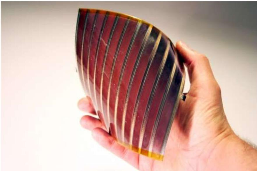
**Figure 1. Dye sensitized solar cells are thin, lightweight and flexible [7]**
