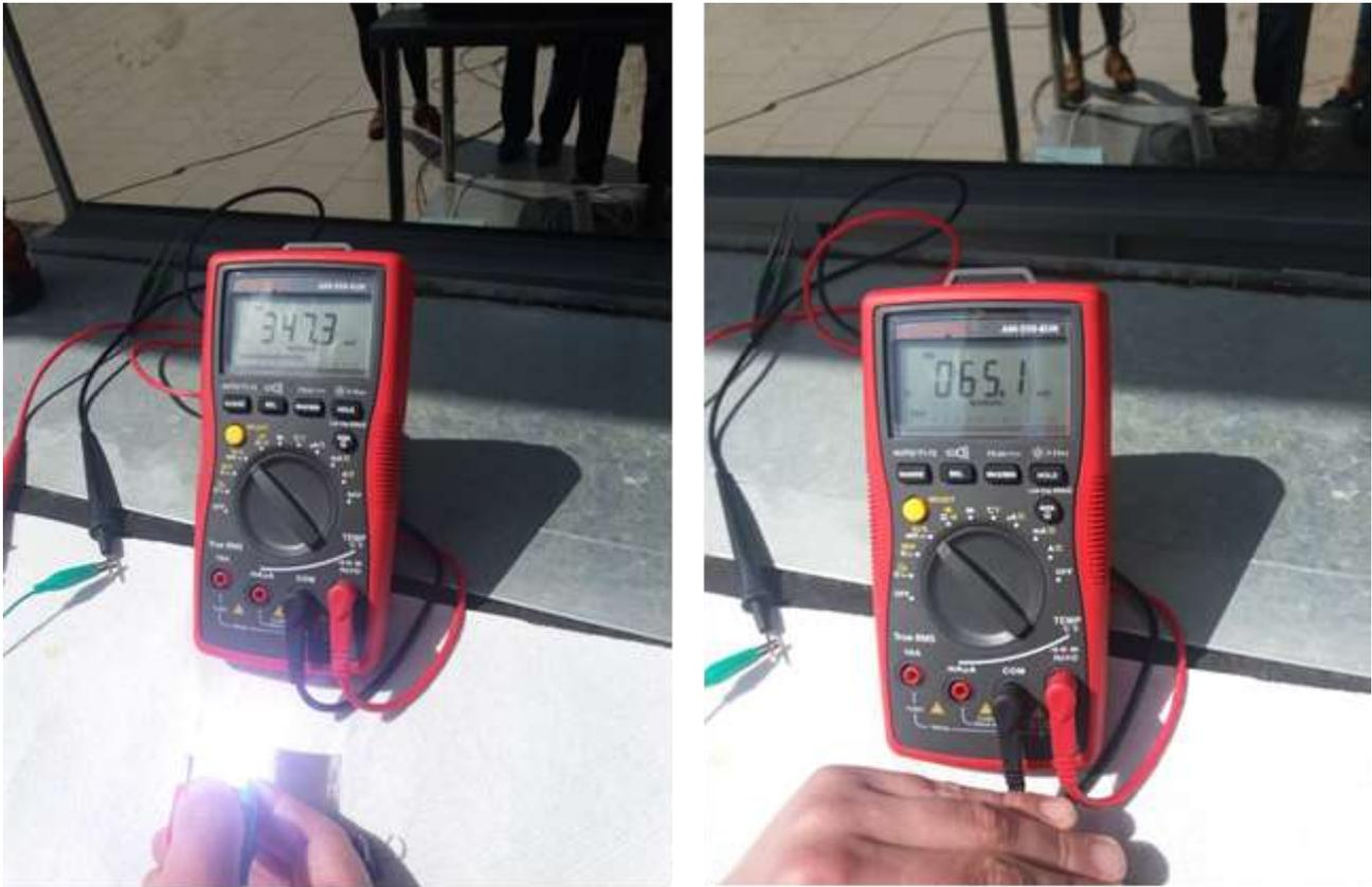
**Figures 12, 13. DSC prototype output measurement, courtesy of INCDTIM Cluj, August 2018. Voltage was measured at 50 to 500 mV, depending on solar radiation and intensity ranged between 50 and 150  $\mu$ A for a 3 by 3 cm cell.**
