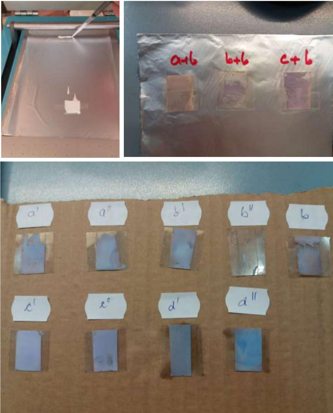
**Figures 9-11. DSC prototype creation, courtesy of INCDTIM Cluj, July 2018. First stage - applying the TiO<sub>2</sub> coating paste evenly with a machine. Second stage - sintering at 150° C and then dipping overnight in an organic blueberry concentrated dye solution. Several tries were necessary for a stable and even coating to be achieved on ITO films**
