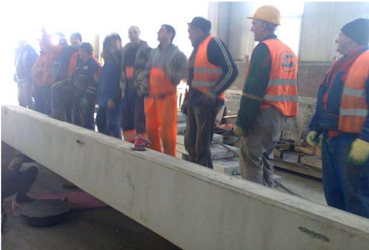
Figure 4. Generation of human induced vibrations for the seating decks
