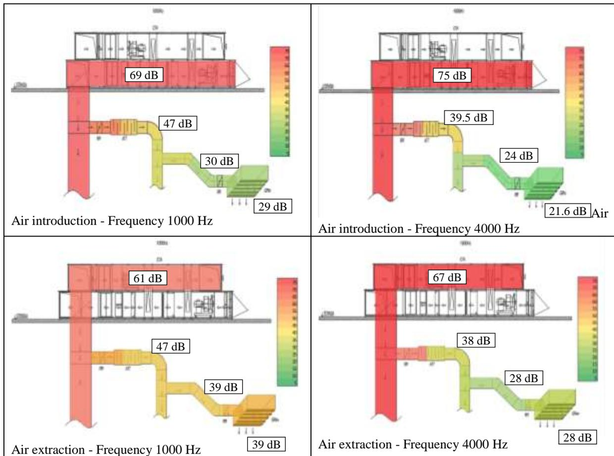
Figure 8. Noise maps for introduction/extraction air at 1000 Hz and 4000 Hz
