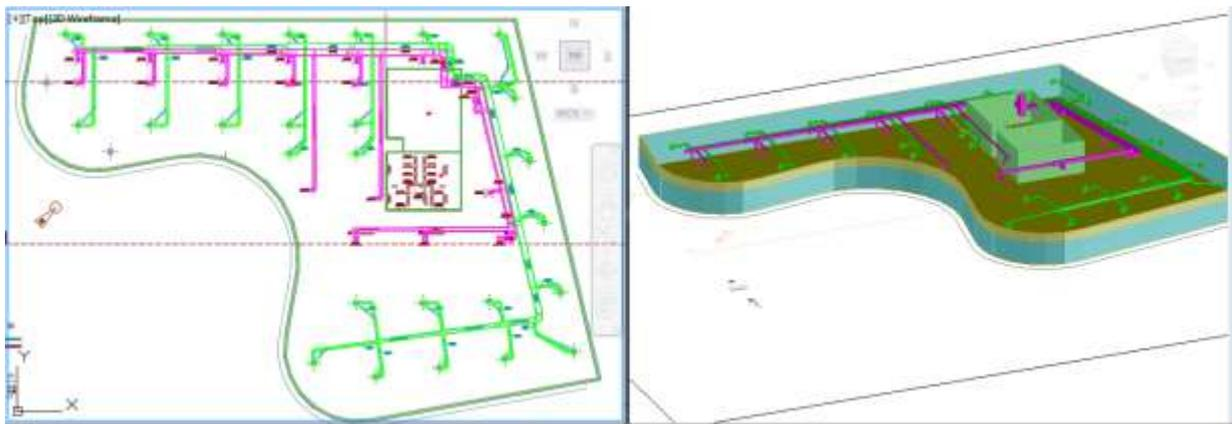
Figure 4. HVAC system distribution (inlet/outlet) and 3D model for noise determination
