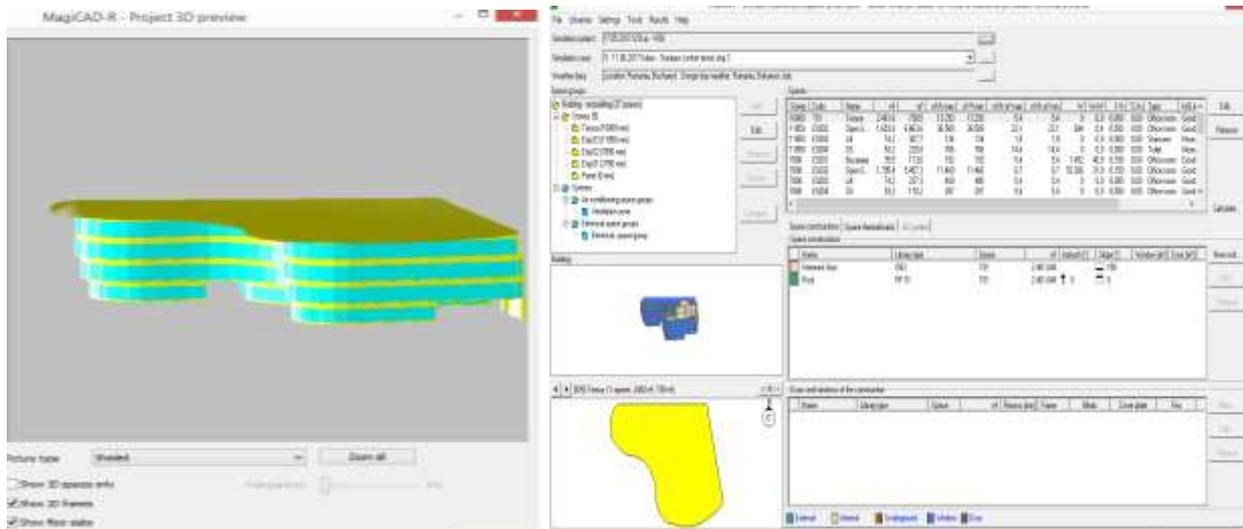
Figure 2. a) Presentation of the 3D model of the building in MagiCAD Room b) Import into Riuska of the 3D model
