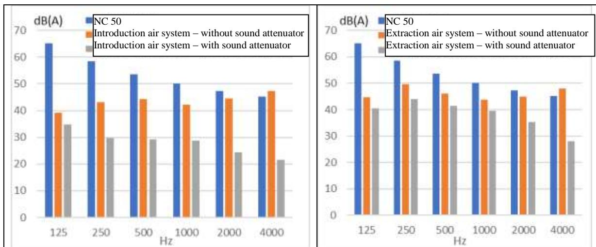
Figure 7. Sound pressure levels [dB] for inlet air diffusion and extraction air
