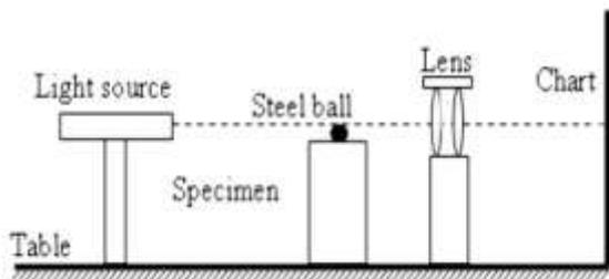
Figure (1) layout of plastic shrinkage apparatus.
