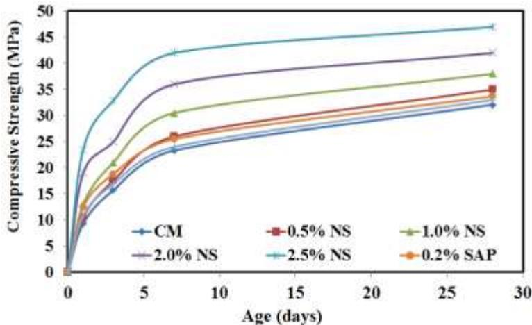
Figure (10) the relation between compressive strength and age (days) for different mixes.
