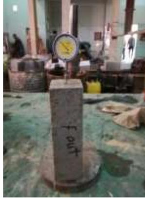
Figure (3) Apparatus for measuring drying shrinkage.
