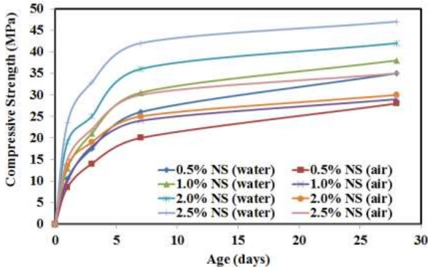
Figure (11) the relation between compressive strength and age (days) for mix containing different percent of Nano-silica with different curing.
