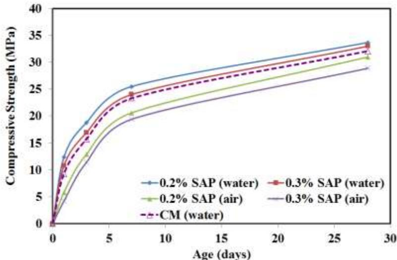
Figure (12) the relation between compressive strength and age (days) for mix containing different percent of SAP with different curing.
