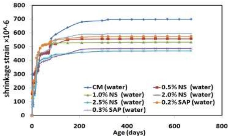
Figure (7) relation between drying shrinkage strain and age for mixes with different percent of Nano-silica and super absorbent polymers.
