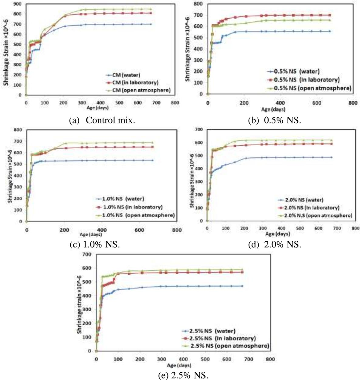
Figure (8) relation between drying shrinkage strain and age (days) for mix with Nano-silica as an addition of cement content at different curing conditions.
