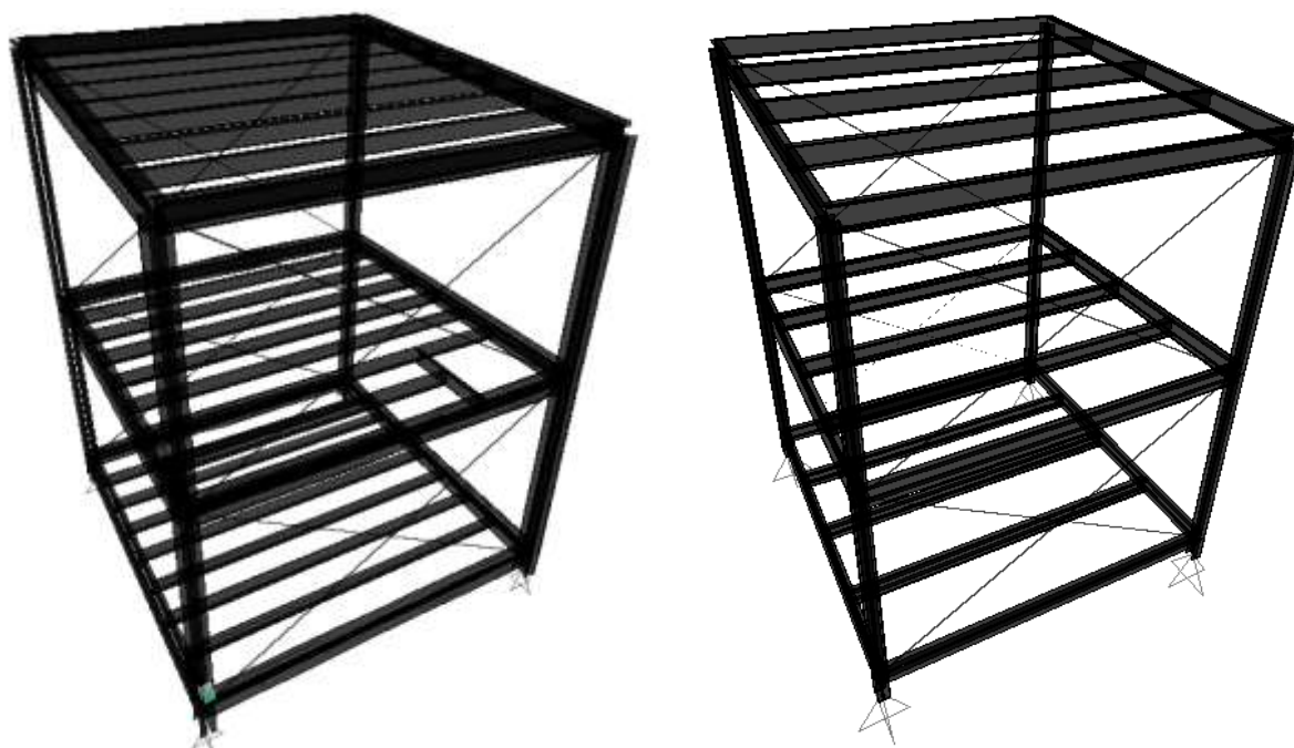
Figure 1 – Load bearing structure using cold formed profiles (left) and hot rolled profiles (right) (source: extruded 3D view, SAP2000 Structural Software for Analysis and Design[16])
