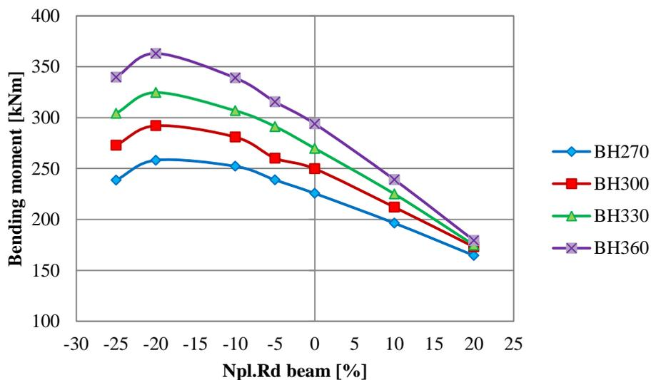
Figure 7. M-N interaction diagrams for specimens with different beam height
