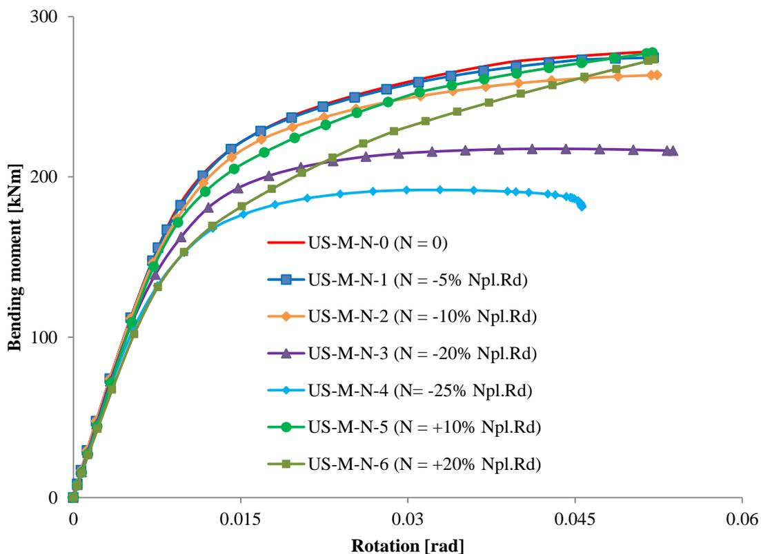
Figure 4. M- $\Phi$  curves of the US specimens subjected to a combination of bending and axial forces
