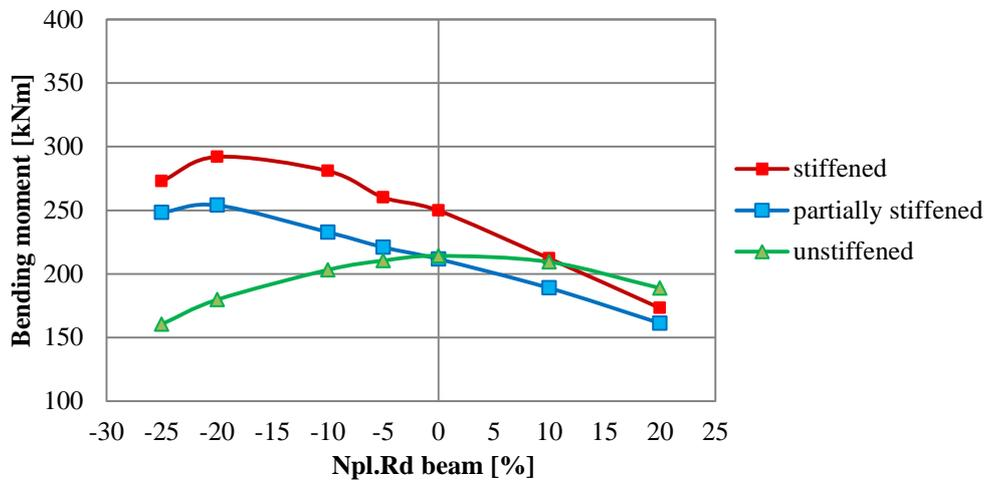
Figure 3. M-N interaction diagram for the studied connection
