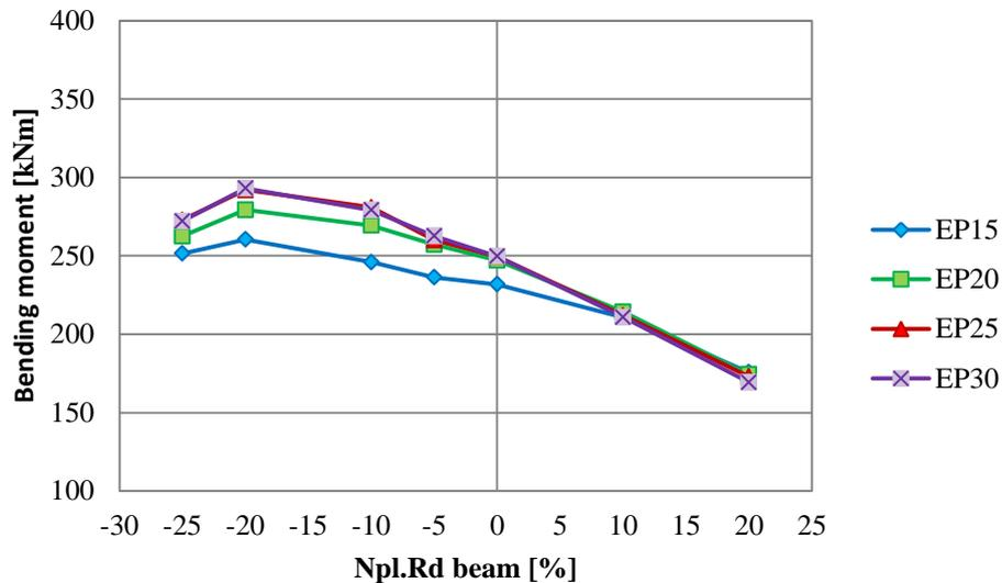
Figure 6. M-N interaction diagrams for specimens with different end-plate thicknesses
