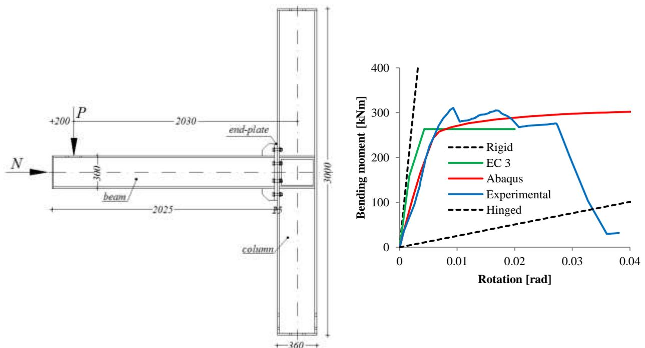
Figure 1. a. Connection mechanical model; b.  $M-\Phi$  curves of the connection
