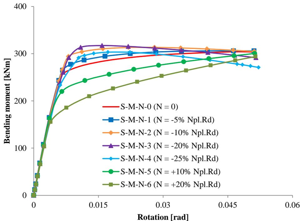
Figure 2. M- $\Phi$  curves of the S specimens subjected to a combination of bending and axial forces
