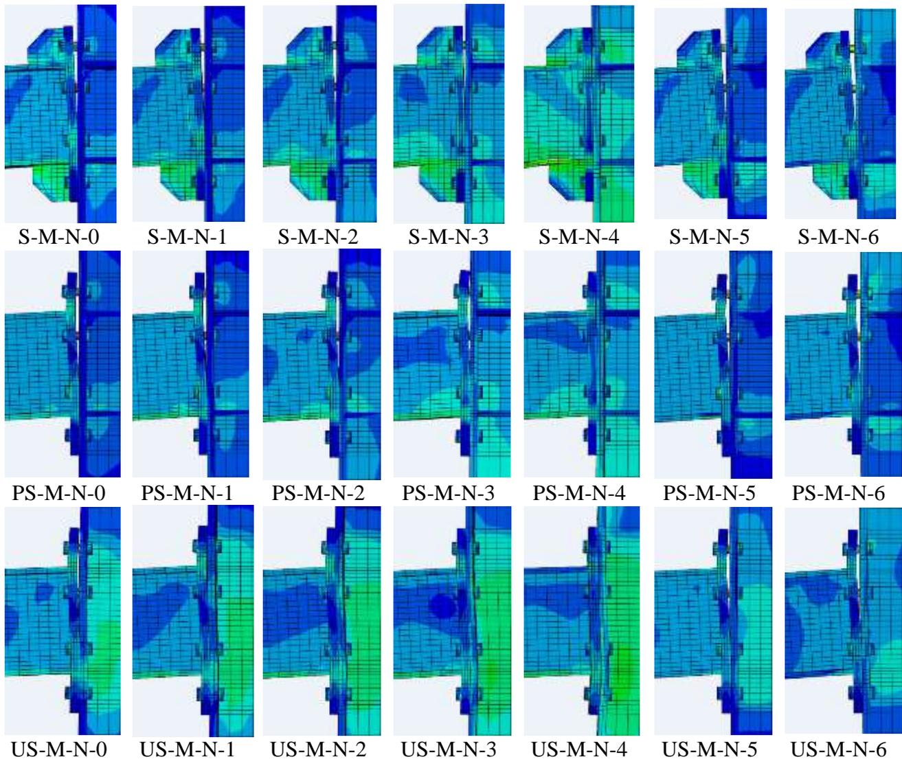
Figure 5. Von Mises stress distribution in the connection area
