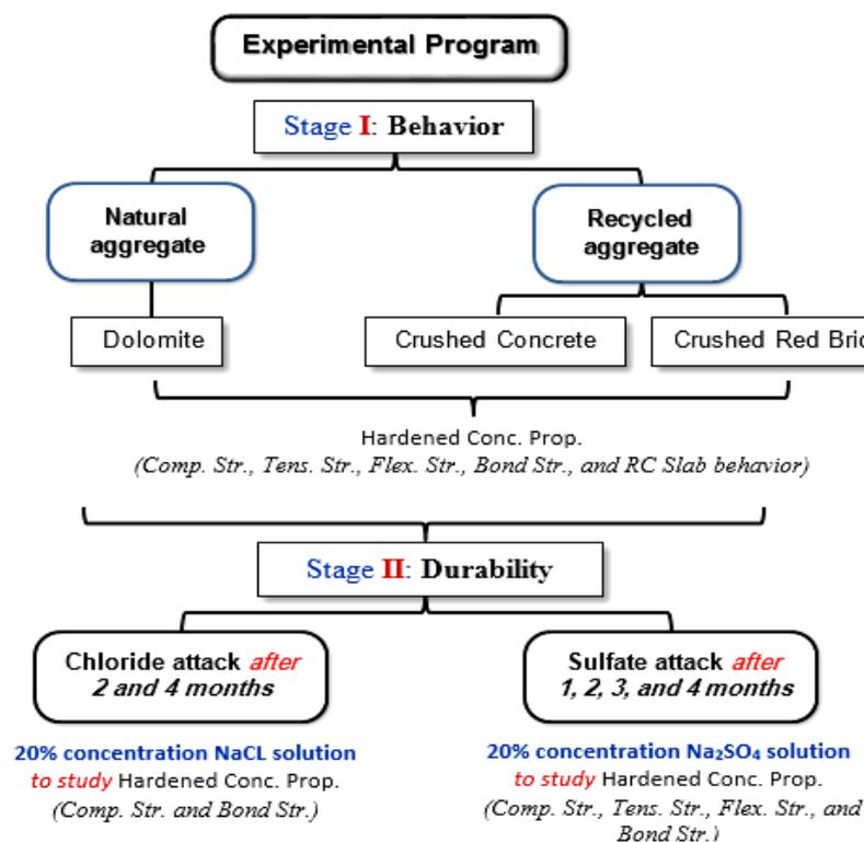
**Fig. 1:** Flow chart of the experimental program.
