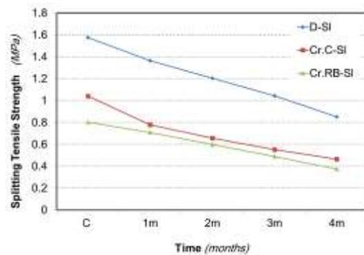
Fig. 20: Effect of sulfate on splitting tensile strength.
