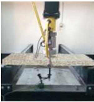
**Fig. 9:** Hydraulic jack and the loading frame of slab samples.
