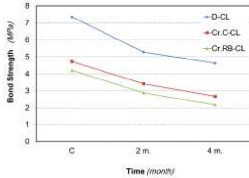
Fig. 18: Effect of chlorides on bond strength.
