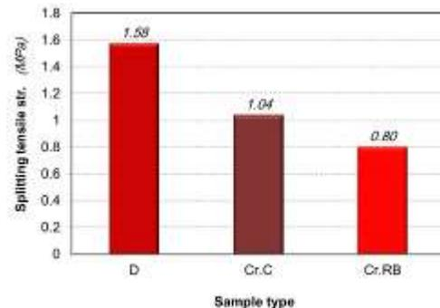
Fig. 12: Splitting tensile strength of control samples.
