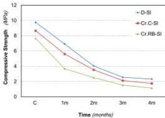
Fig. 19: Effect of sulfate on compressive strength.
