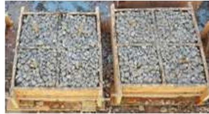
**Fig. 5:** Pervious concrete cube samples.
