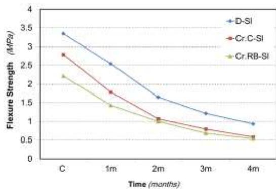
Fig. 21: Effect of sulfate on flexure strength.
