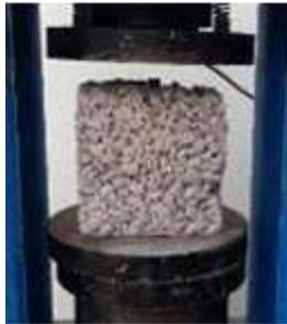
**Fig. 2:** Compressive strength test.
