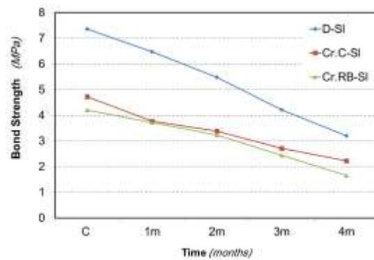
Fig. 22: Effect of sulfate on bond strength.
