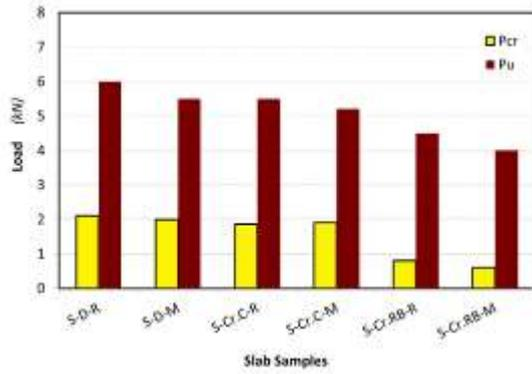
Fig. 15: Initial cracking load and ultimate loads for tested slabs.
