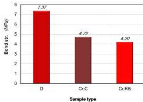
Fig. 14: Bond strength of control samples.
