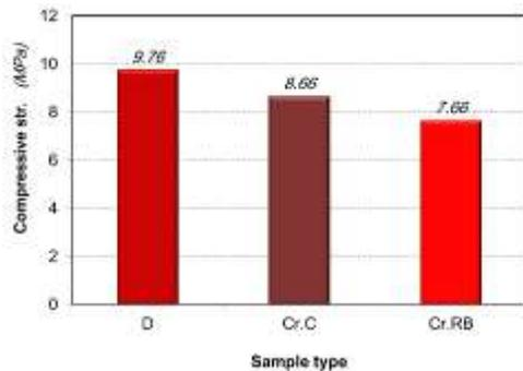
Fig. 11: Compressive strength of control samples.
