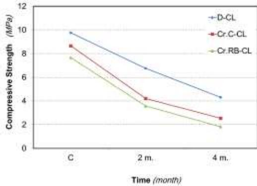
Fig. 17: Effect of chlorides on compressive strength.
