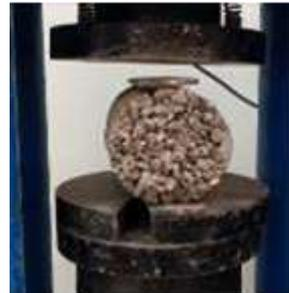
**Fig. 3:** Splitting tensile strength test.
