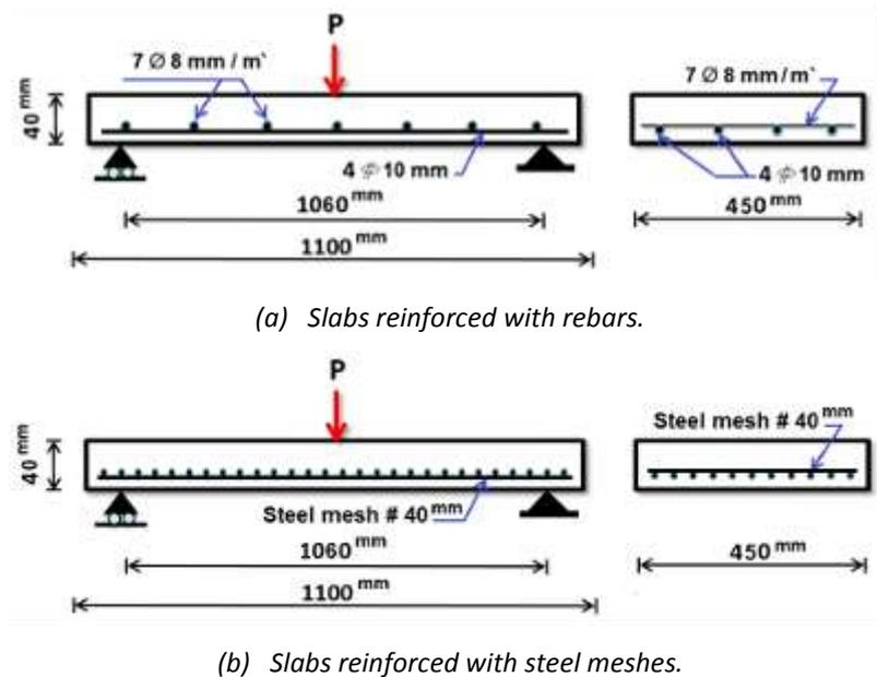
**Fig. 8:** Details and reinforcement of tested slab samples.
