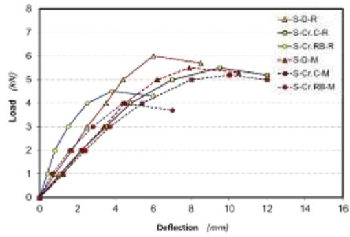
Fig. 16: Load-deflection relationships for tested slabs reinforced with rebars or with meshes.
