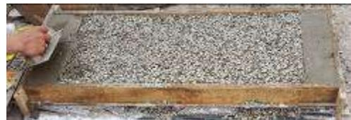
**Fig. 7:** Preparing the supports at the lower surface of slab samples.
