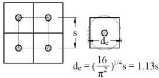
Figure 3. Unit cell diameter for square pattern arrangement of the inclusions [2]
