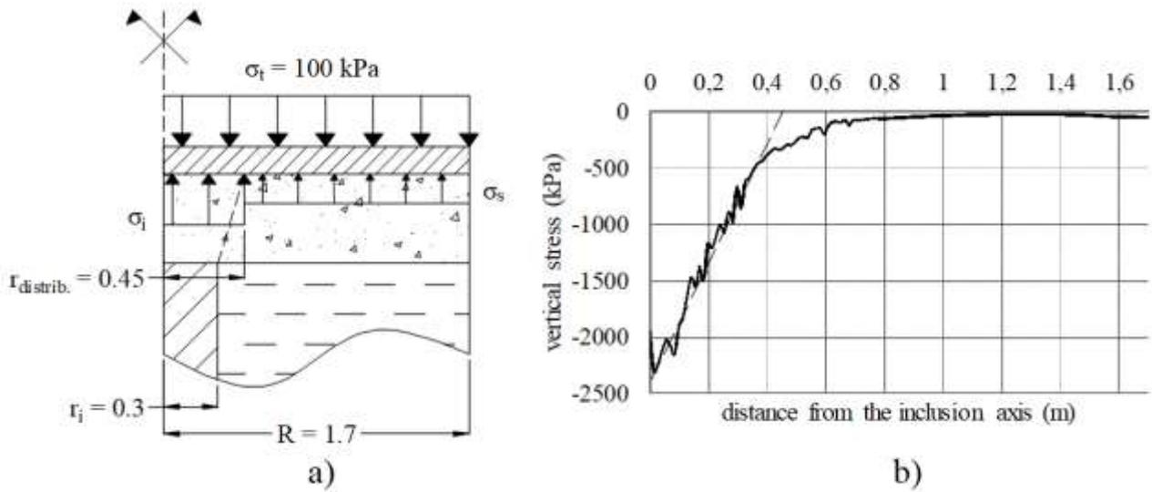
Figure 5. Analytical calculation scheme after Bohn 2016 [10] (a) and vertical stress distribution on the base of the foundation from the finite element analysis (b)
