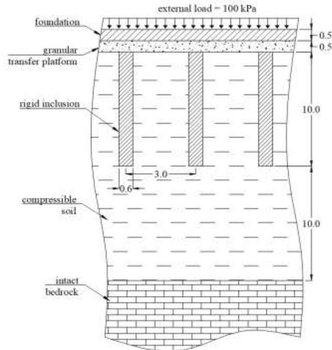
Figure 1. Schematic representation of the analyzed situation (not scaled)
