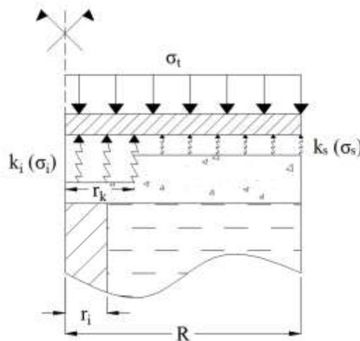
Figure 6. Elastic Winkler model with two reaction coefficients [7]
