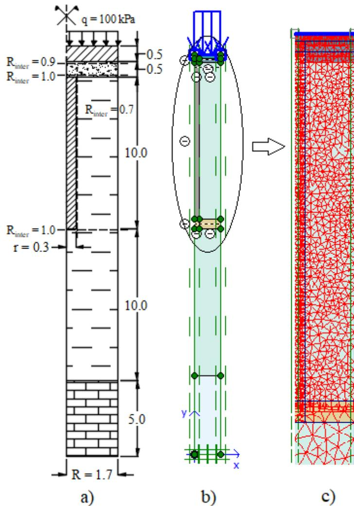
Figure 2. a) schematic representation of the unit cell model (not scaled); b) axisymmetric unit cell model in Plaxis 2D; c) discretization of the unit cell model in Plaxis 2D
