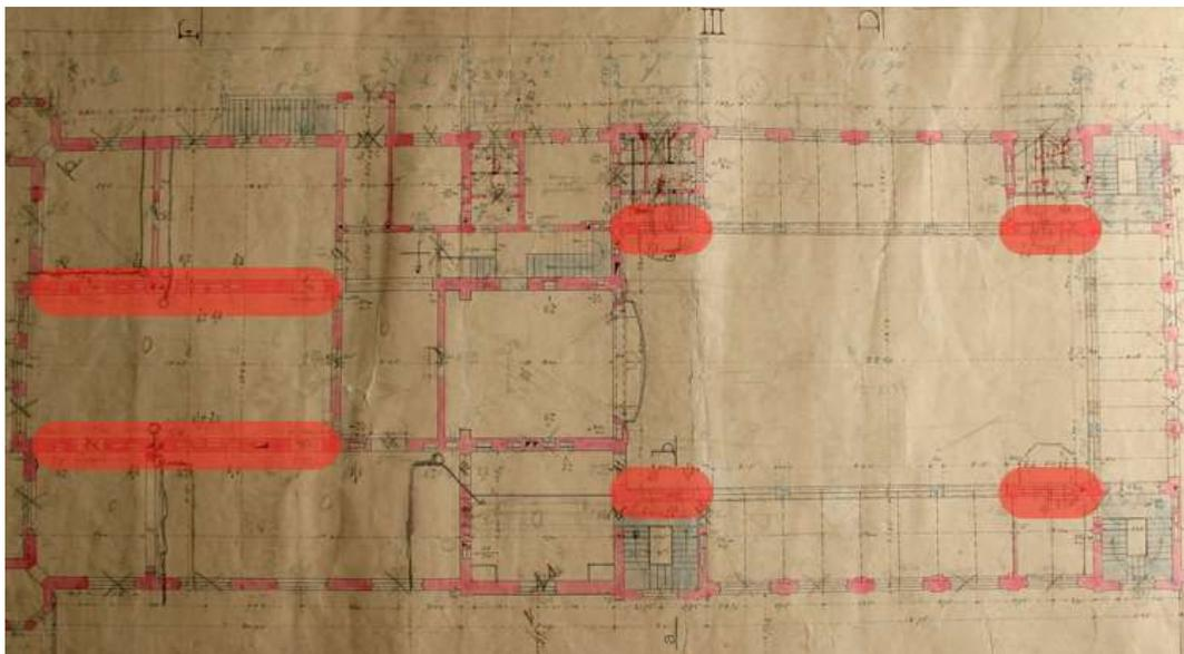
Figure 6 - Ventilation tunnels marked disposal marked on plan - original plan 1895 -
