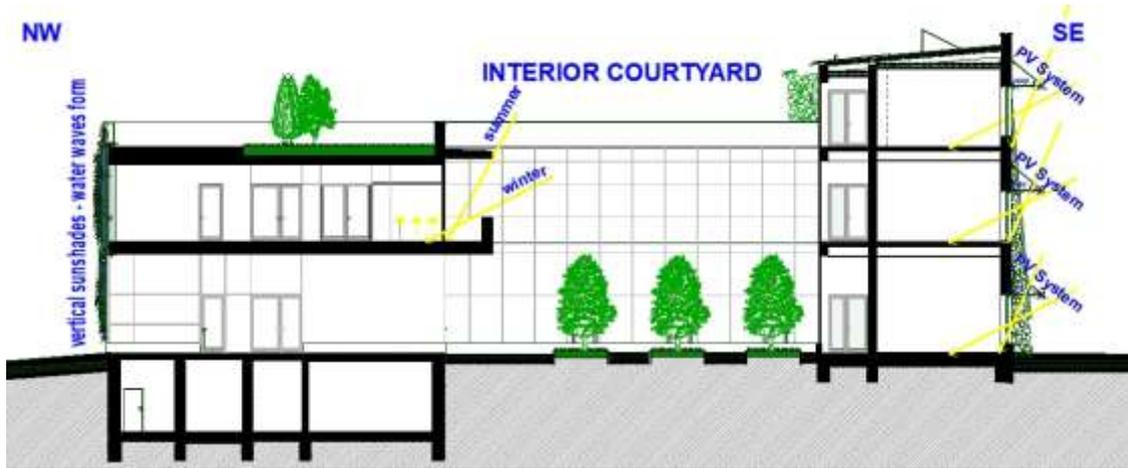
Figure 4. Section with metal structures designed for actual horizontal sunshades and a potential future photovoltaic system on the South-East elevation and vertical sunshades on water waves form on North West elevation (2)
