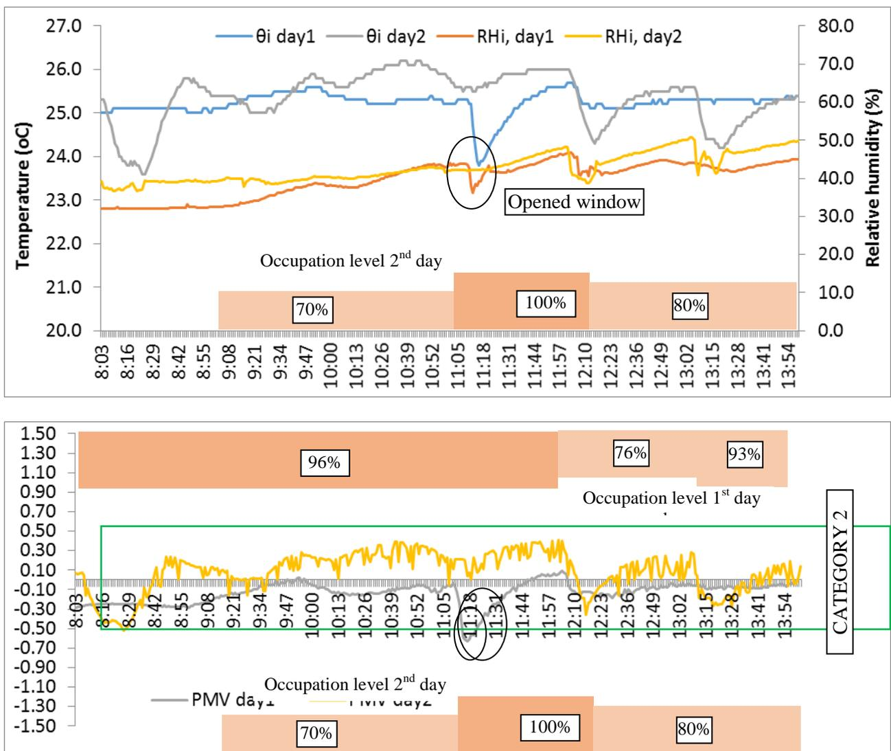
Figure 2. Analysis of thermal comfort for the non-ventilated room
