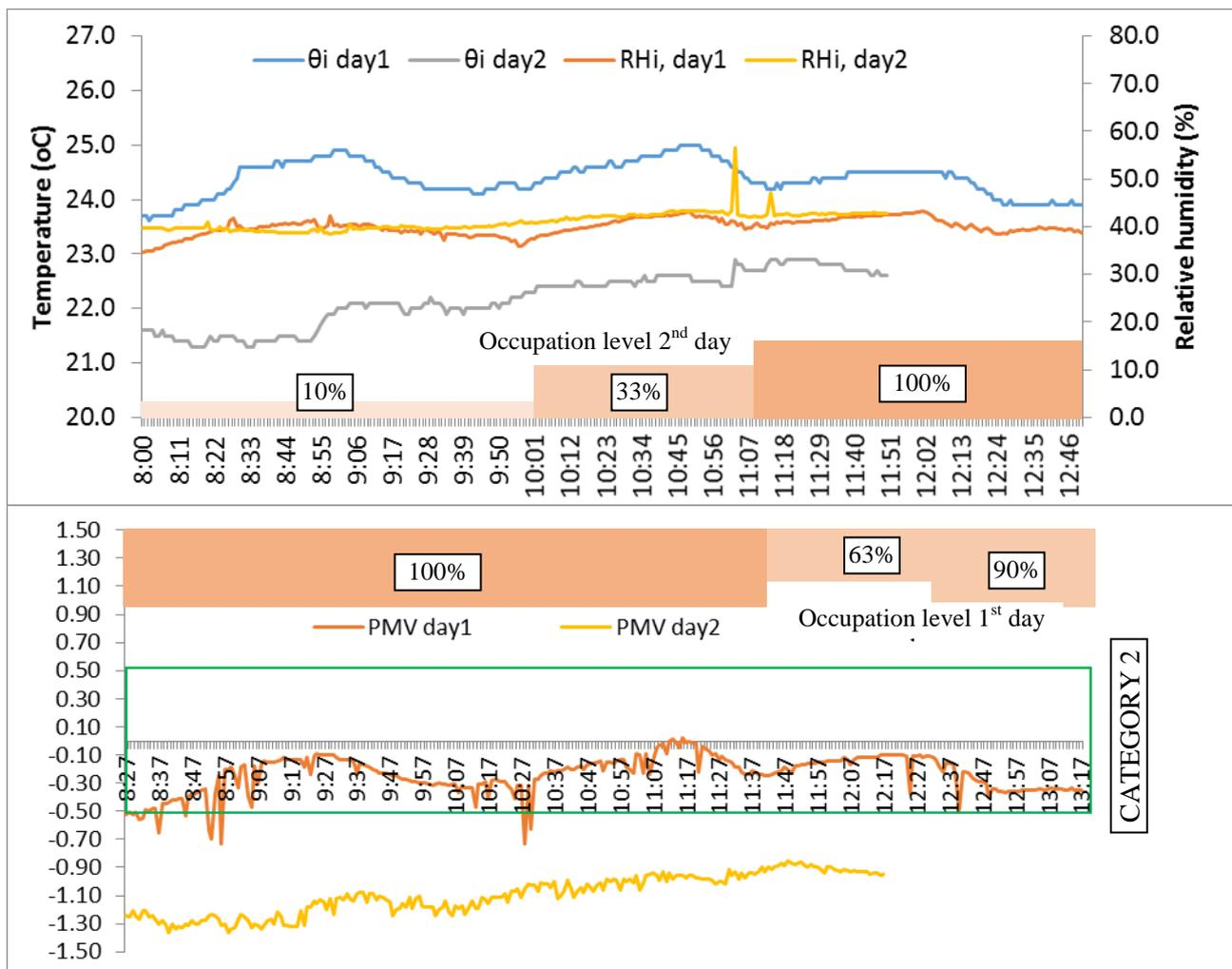
Figure 3. Analysis of thermal comfort for the ventilated room
