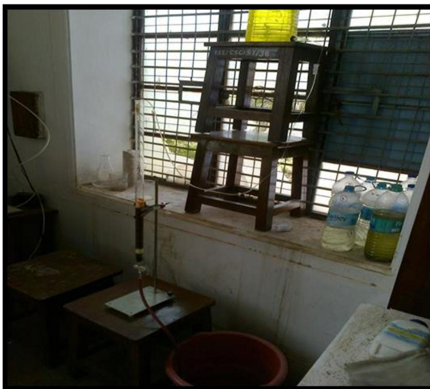
Figure 10. Column Model Used for Cr Adsorption
