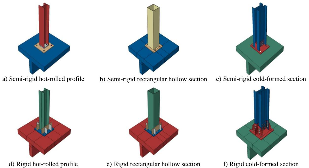
Figure 6: Semi-rigid and rigid base connections
