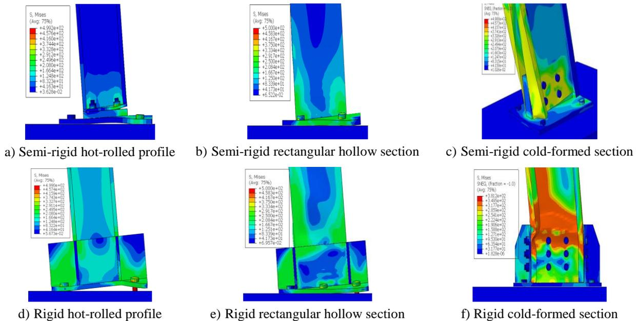
Figure 8. Plastic strains in the semi-rigid and rigid based connections
