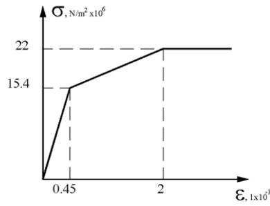
Figure 7. Elastic-plastic model of concrete [6]
