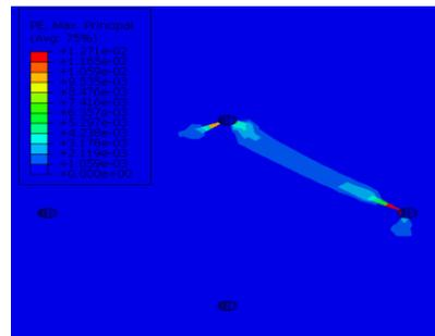
Figure 9. Strains in concrete on bolt hole
