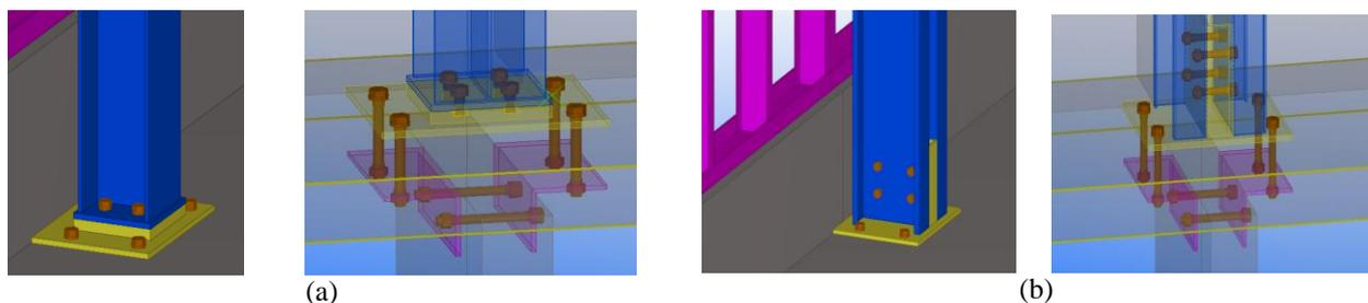
Figure 5. Column-base connection details case 1 and case 3 respectively
