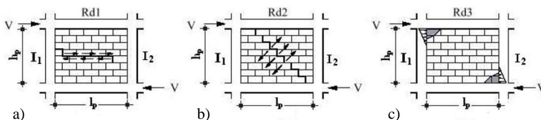
Figure 6. Failure modes of the infill wall panel
