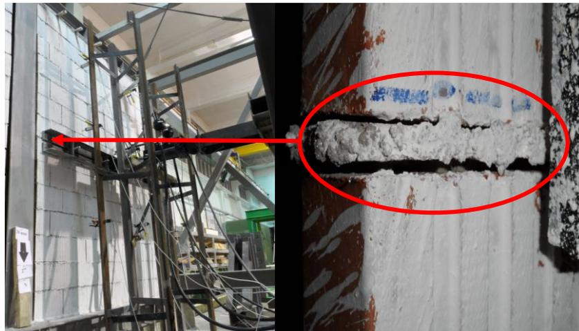
Figure 12. Experimental setup and opening of horizontal crack in MW1
