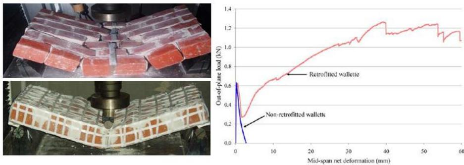
Figure 9. Failure patterns of the tested masonry wallets and out-of-plane load variation [18]
