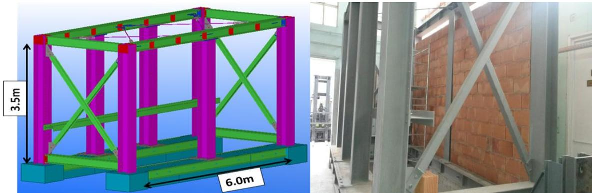
Figure 7. Design and construction of the experimental stand
