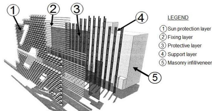
Figure 6. Proposal of a 4 layer exterior consolidation method
