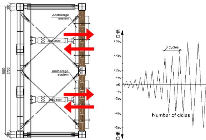
Figure 10. Testing procedure and loading protocol
