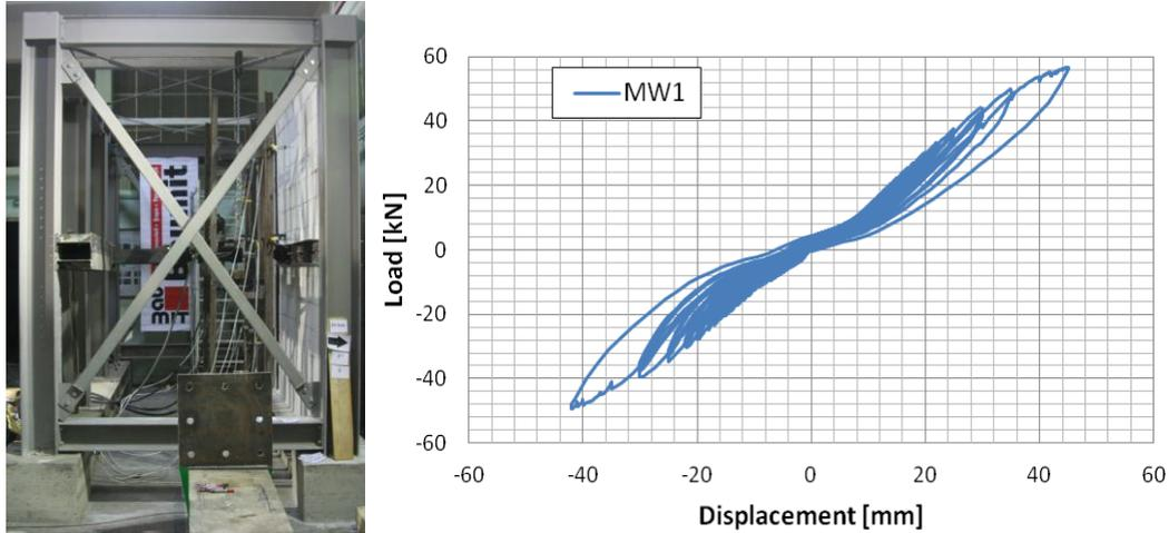
Figure 11. Experimental setup and load-displacement diagram for MW1
