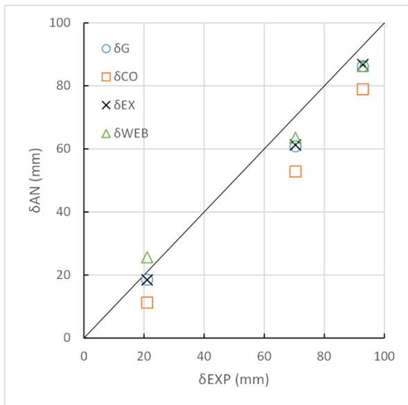
Figure 9. Analytic deflection  $\delta_{AN}$  versus experimental deflection  $\delta_{EXP}$ , at maximum capacity (ULS).
