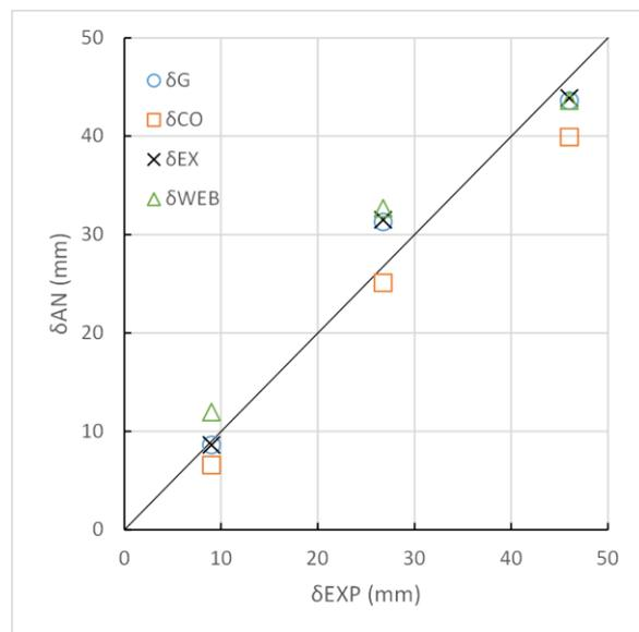
Figure 10. Analytic deflection  $\delta_{AN}$  versus experimental deflection  $\delta_{EXP}$ , at 50% of the maximum capacity.
