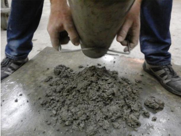
Figure 1. Slump-flow for preliminary mix
