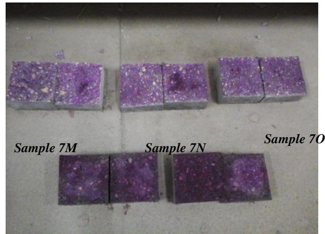
Figure 9. Carbonation depth.
