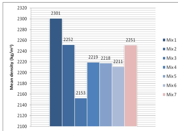
Figure 6. Density of the concrete mixes.
