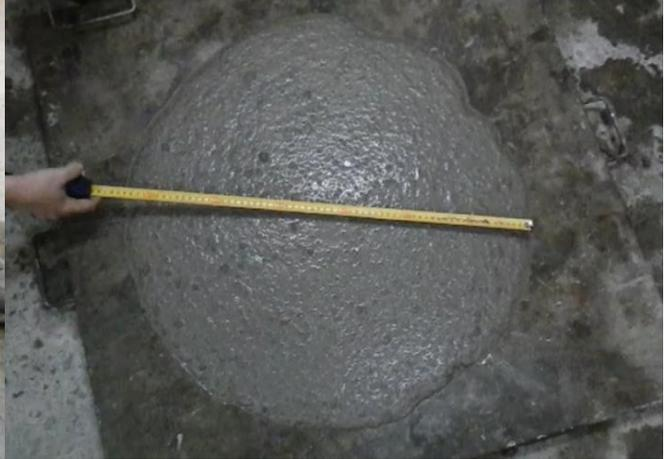
Figure 2. Slump-flow for mix 7
