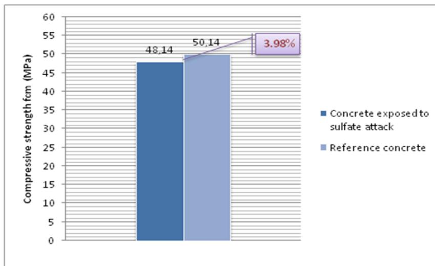
Figure 8. Loss of compressive strength due to the sulfate attack.
