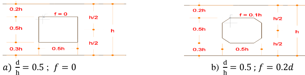
Figure 6. Variation of chamfered joints dimensions.
