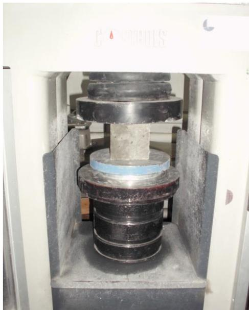
Figure 2. Compression test
