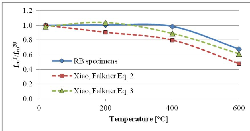
Figure 6. Regression for compressive strength
