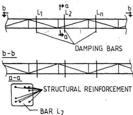
Fig.2. Passive damper in the form of lamella
