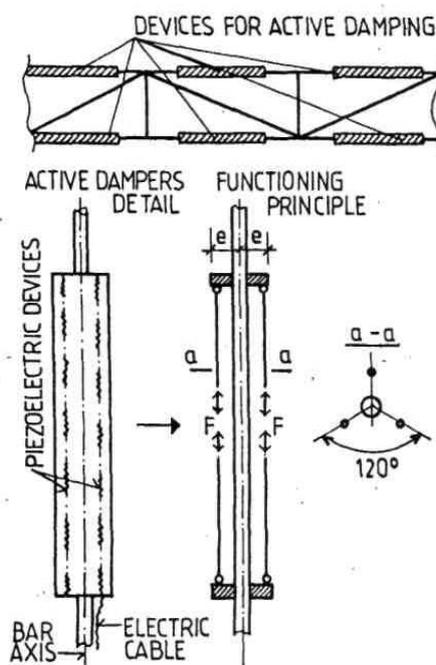
Fig.5. Active damper with piezoelectric crystals
