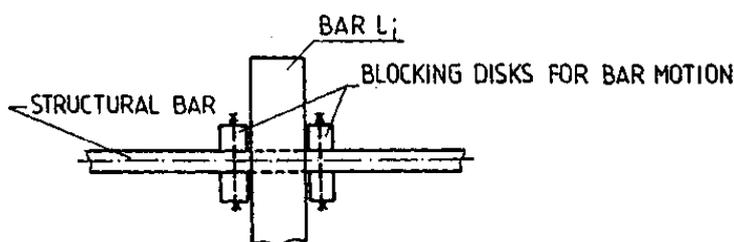
Fig.4. Connecting the bars
