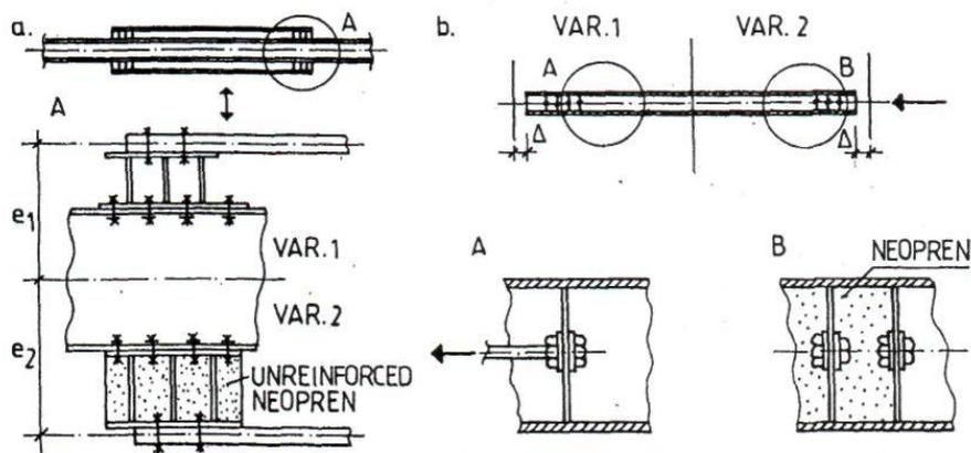
Fig.1. Passive dampers
