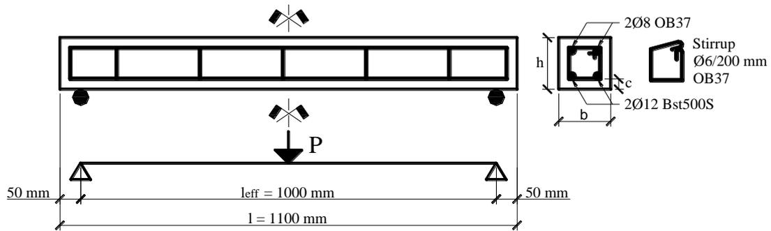
Figure 1. Reinforcement detailing and set-up test
