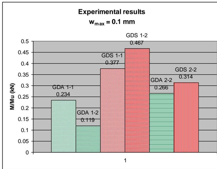
Figure 6. Experimental bending moment at  $w_{max} = 0.1$ mm / ultimate moment
