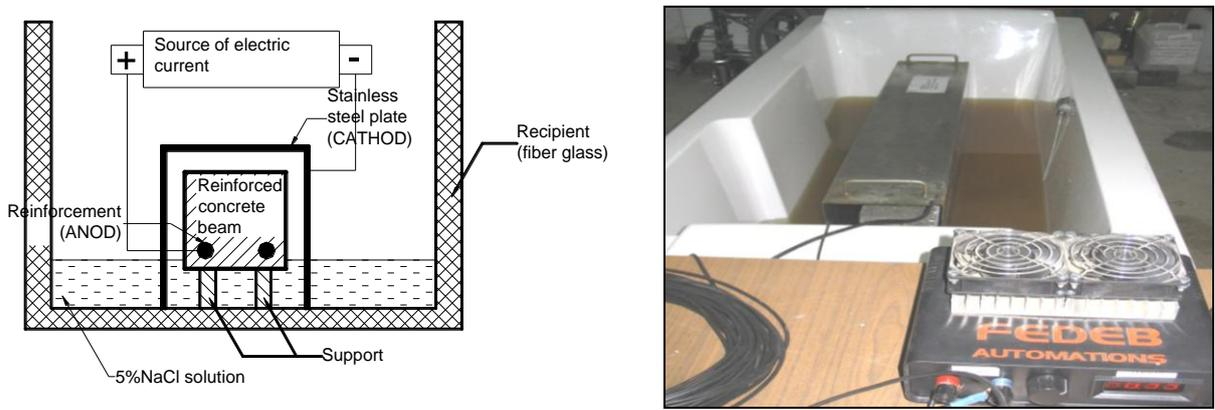
Figure 3. a. Schematic view of the corrosion process; b. Corrosion equipment
