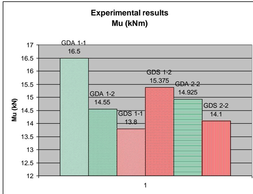
Figure 8. Experimental ultimate bending moments
