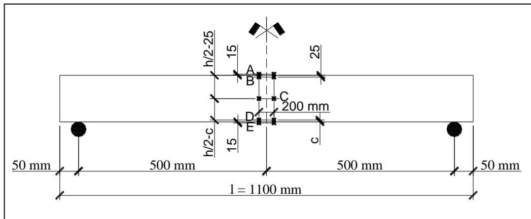
Figure 2. Placement of the measurement devices
