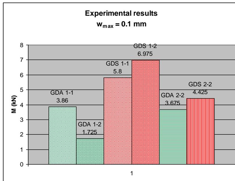
Figure 5. Experimental bending moment at  $w_{\max} = 0.1\text{mm}$
