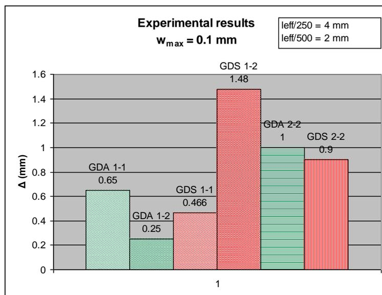
Figure 7. Experimental vertical deformations at  $w_{max} = 0.1$ mm
