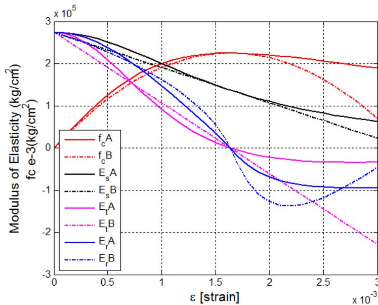
Fig. 2. A: Todeschini model, B: Hognestad model, s: secant modulus, t: tangent modulus, r: reduced modulus of elasticity
