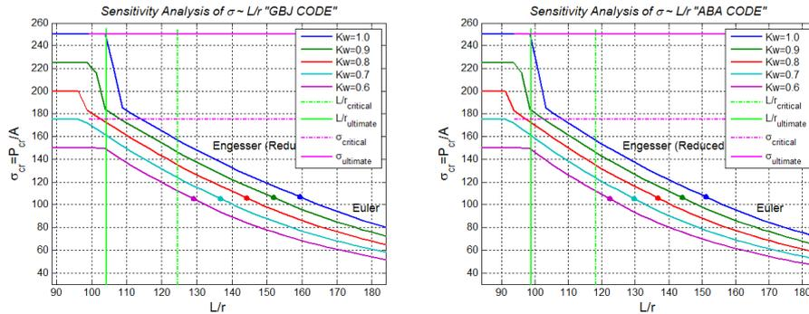
Fig. 16.  $P_u/P_0=1, \rho=2, e=0, I_m=0.65I_g$ , left GBJ code, right ABA code.  $K_w=0.6$  to 1
