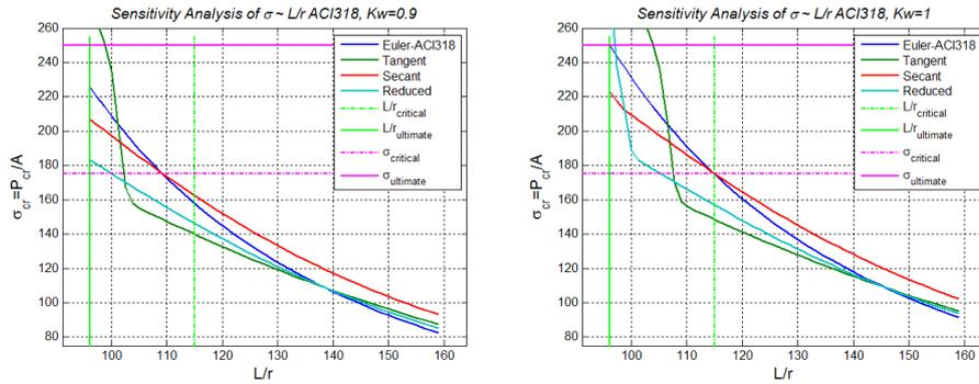
Fig. 12. Buckling stress versus slenderness for various types of modulus theories and ACI-318 code.  $I=1.0 I_g$ , left:  $K_w=0.9$ , right  $K_w=1.0$
