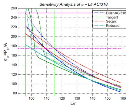
Fig. 13. Buckling stress versus slenderness for various types of modulus theories and ACI-318 code.  $I=1.0 I_g$ , (-)  $K_w=0.9$ , (-)  $K_w=1.0$
