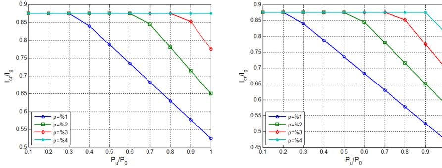
Fig. 8. Cracked moments of inertia of compression and flexural members according to different reinforcement ratios, left  $e=0, M_u=0$ , right  $e=5\%, M_u=0.05 \cdot h \cdot P_u$
