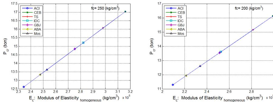
Fig. 10. Elastic modulus change with critical load according to different codes, (left  $K_w=1$ , right  $K_w=0.8$ )
