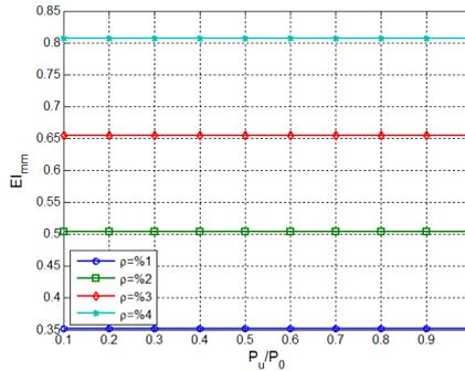
Fig. 9.  $EI_{eff}$  according to different reinforcement ratios ( $\beta_d=0, C_t=2.2, ACI318$ )
