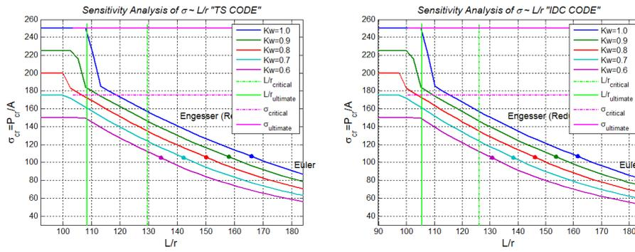
Fig. 15.  $P_u/P_0=1, \rho=2, e=0, I_m=0.65I_g$ , left TS code, right IDC code.  $K_w=0.6$  to 1
