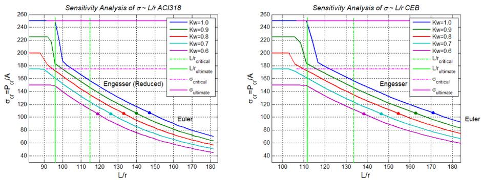
Fig. 14.  $P_u/P_0=1$ ,  $\rho=2\%$ ,  $e=0$ ,  $I_m=0.65 I_g$ , left ACI code, right CEB code.  $K_w=0.6$  to 1
