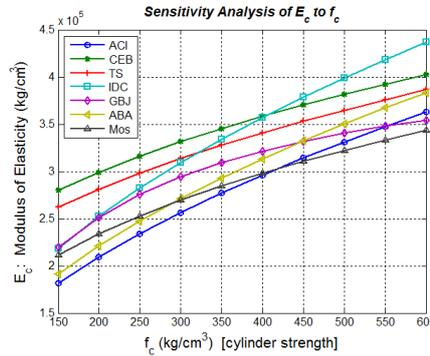
Fig. 6. Relationship curves of elasticity Modulus and various concrete strengths for different design codes,  $K_c=1$
