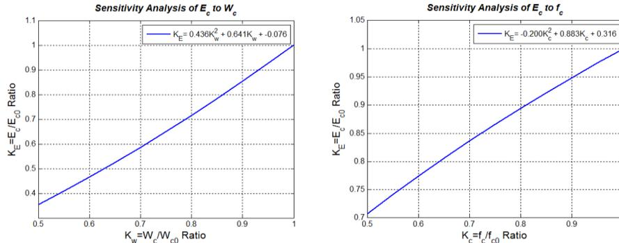
Fig. 3. Sensitivity analysis of  $E_c$  with  $W_c$  and  $f'_c$  according to different  $K_w$  and  $K_c$  ratios
