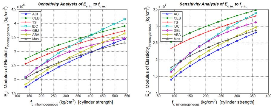
Fig. 7. Relationship curves of elasticity modulus and various concrete strengths for different design codes, left:  $K_c=0.9$ , right:  $K_c=0.6$  [ $K_c=f'_c/f'_{c0}$ ]
