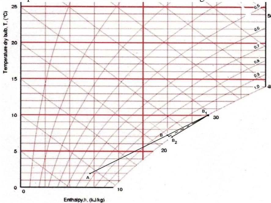
Figure 3. Air treatment process using groundwater
