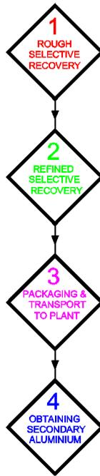
Figure 1. The four stages involved in aluminium recycling.
