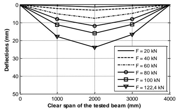
Figure 14. Displacement profile for beam B02-I-2L.
