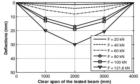
Figure 16. Displacement profile for beam B04-II-2L.
