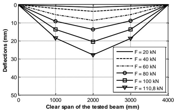
Figure 13. Displacement profile for beam B01-I-1L.
