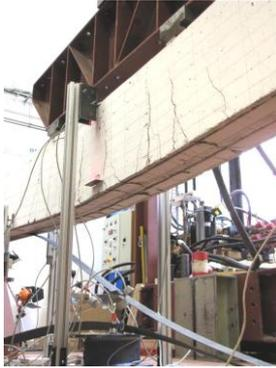
Figure 4. Mid-span debonding of FRP initiated by a flexural crack.
