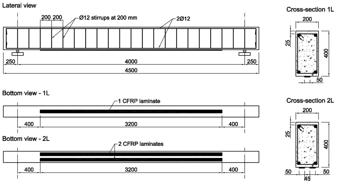
Figure 1. Details of test beams, reinforcement layout and strengthening schemes.
