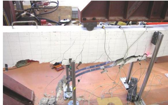
Figure 5. Delamination caused by excessive shear deformation.
