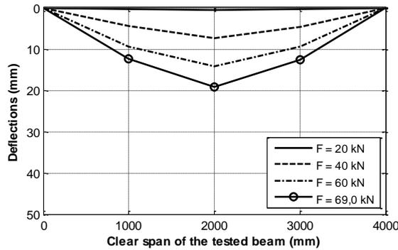
Figure 12. Displacement profile for beam B00-REF.
