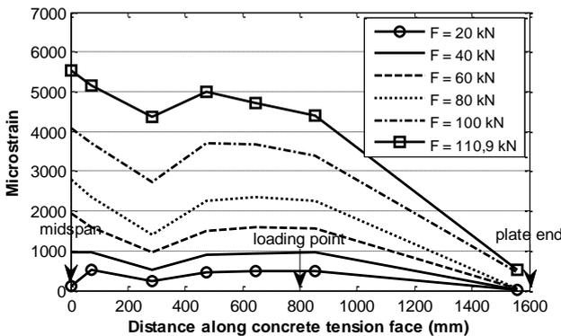
Figure 8. Experimental CFRP strain profile of beam B01-I-1L.
