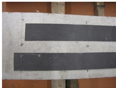
Figure 7. Detail of the ends of the CFRP strips.
