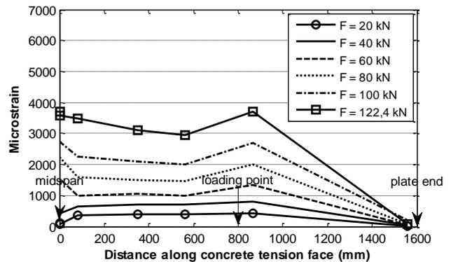
Figure 9. Experimental CFRP strain profile of beam B02-I-2L.
