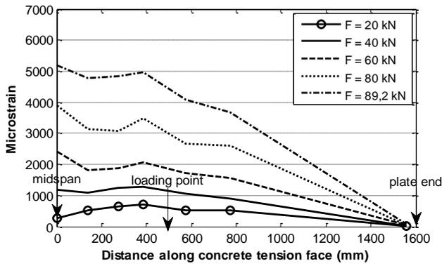
Figure 10. Experimental CFRP strain profile of beam B03-II-1L.
