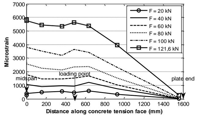
Figure 11. Experimental CFRP strain profile of beam B04-II-2L.
