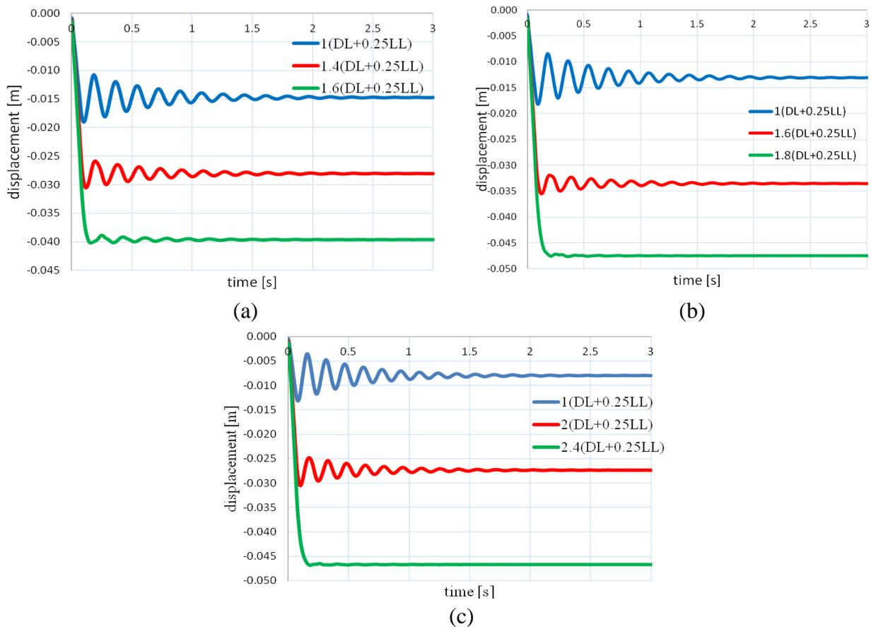
Figure 5. Time-displacement curves of the column-removed point for the models subjected to damage case  $C_4$  for different levels of loading: a) Cluj-model; b) Sibiu-model; c) Bucharest-model.
