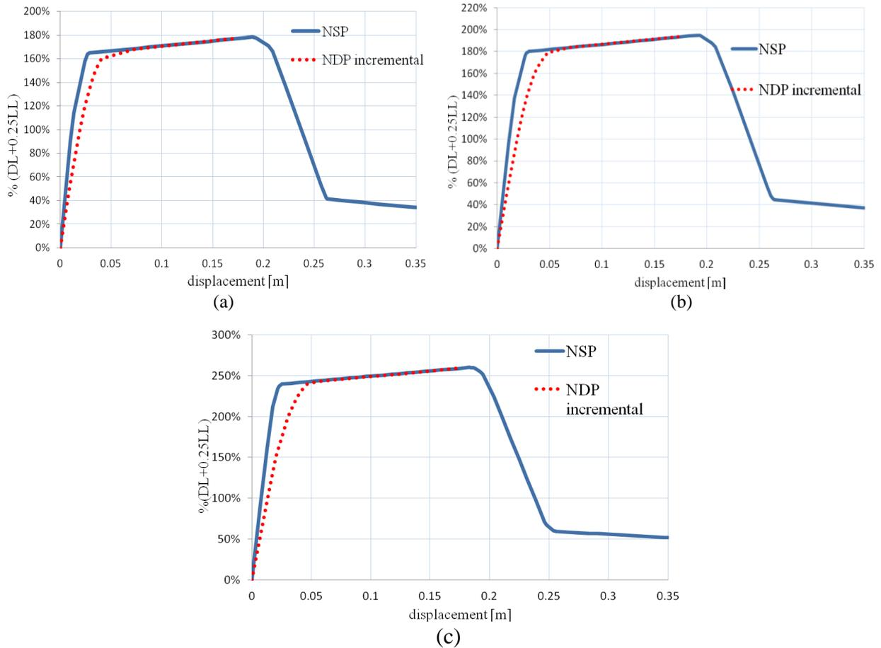
Figure 6. Load-displacement curves obtained with NS and ND incremental analyses for: a) Cluj-model; b) Sibiu-model; c) Bucharest-model, when subjected to interior column removal.
