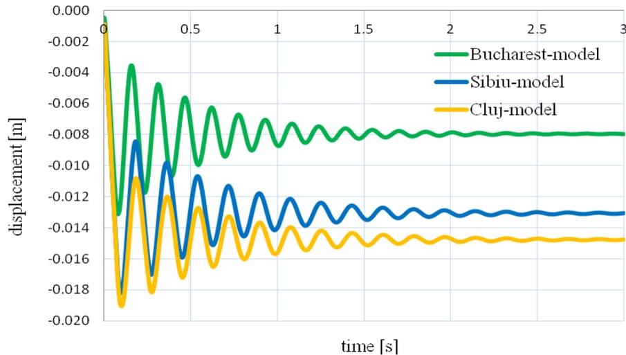
Figure 4. Time-displacement curves of the column-removed point obtained from the nonlinear dynamic analysis.
