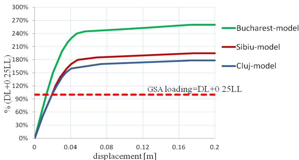
Figure 8. The influence of the seismic design on the potential for progressive collapse of ten-storey structures subjected to the damage case  $C_4$ .
