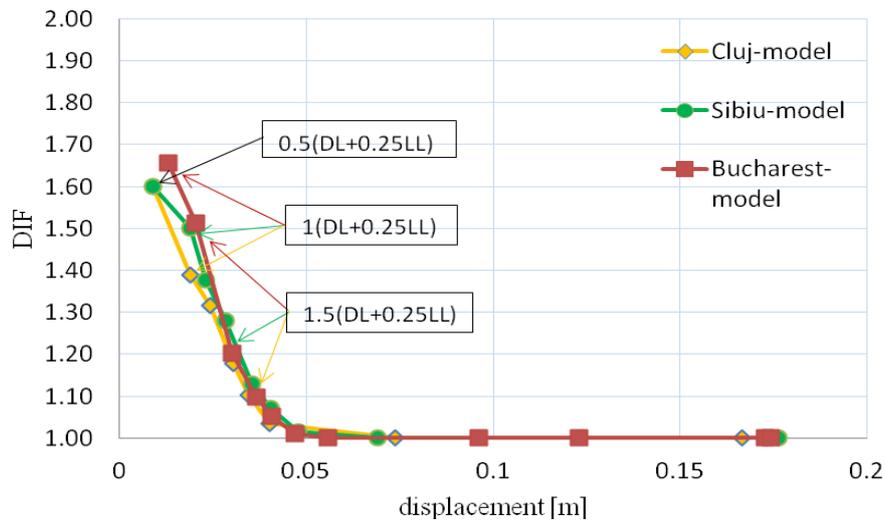
Figure 7. The estimated values of the dynamic increase factor (DIF) based on the capacity curves of the models subjected to the damage case C<sub>4</sub>.
