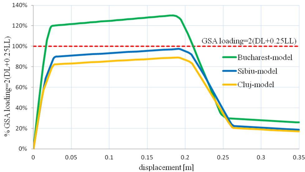
Figure 3. Load-displacement curves obtained from the nonlinear static analysis.
