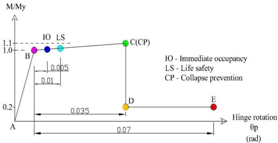
Figure 2. Plastic hinge model.
