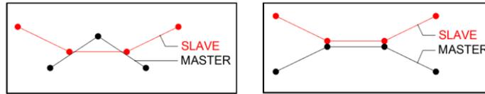
Figure 5. Master/slave surfaces. Node to surface (left side), node to node contact (right side) [9].
