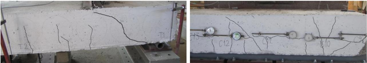
Figure 6. The cracks positions on the lateral and transversal side of the element DG3
