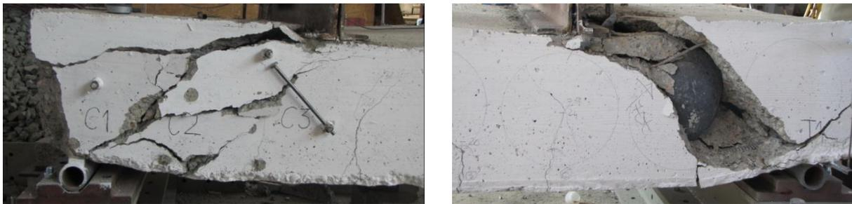
Figure 7. Breaking moment – element DG3
