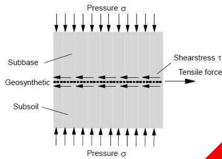
Figure 1: Reinforcement function of geosynthetics
