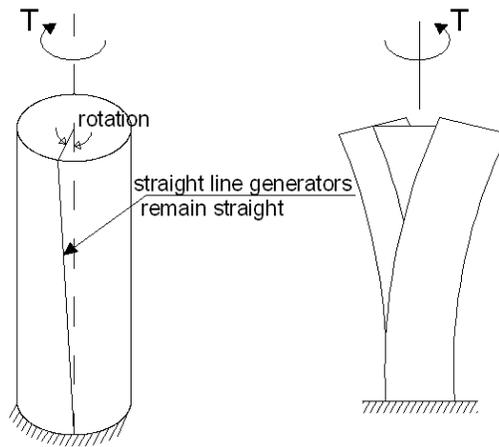
Figure 1. a) St Venant torsion b) warping torsion [2]
