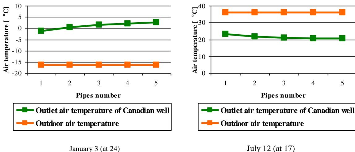
Figure 5. The influence of the number of pipes on the air temperature at the exit from the Canadian well for a cold winter day and a hot summer day.
