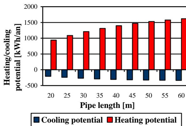
Figure 7. The influence of pipe length upon heating/ cooling potential
