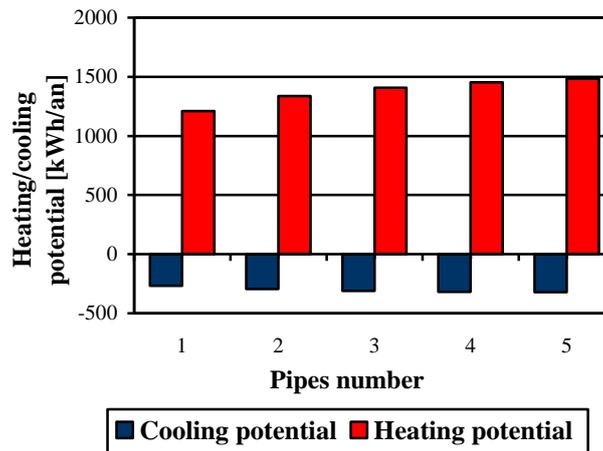
Figure 6. The influence of number of pipes upon heating/ cooling potential
