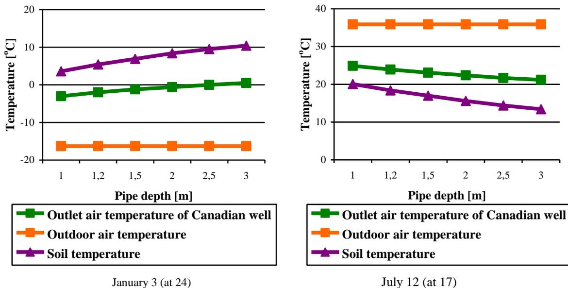
Figure 9. The influence of the mounting depth upon soil temperature and of exit air from the well during a cold winter day and a warm summer one
