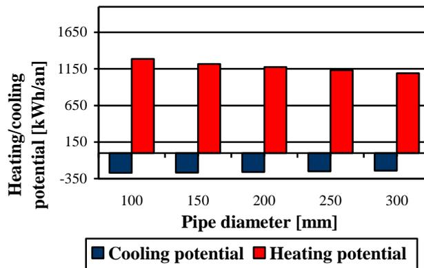
Figure 8. The influence of pipe diameter upon the heating/ cooling potential
