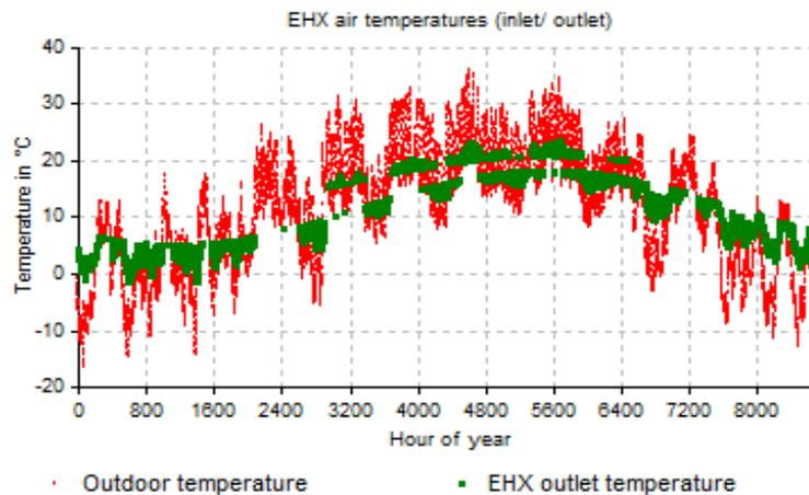
Figure 3. The annual variation of external air temperature and the annual variation of air temperature at the exit from the Canadian well [13]
