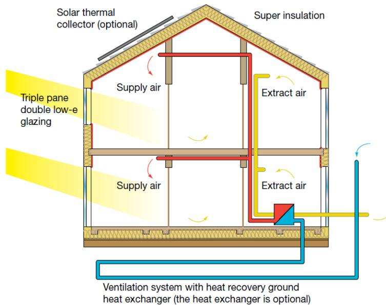
Figure 1. Equipping a passive house with air to air heat exchanger and Canadian well [5]
