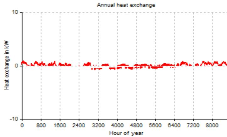
Figure 4. The annual variation of heat flow exchanged by the Canadian well with the soil [13]
