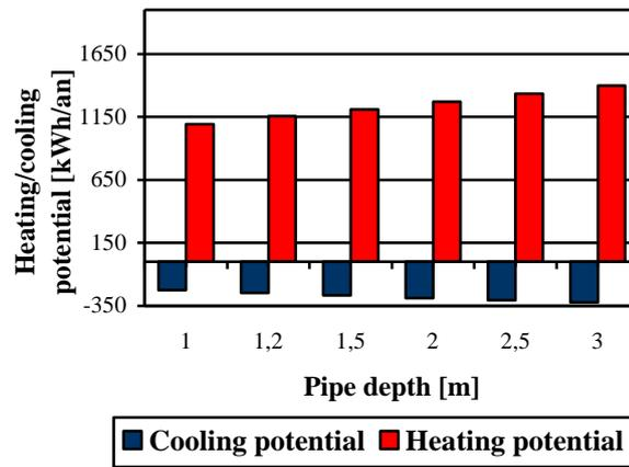
Figure 10. The influence of pipe depth upon the heating/cooling potential
