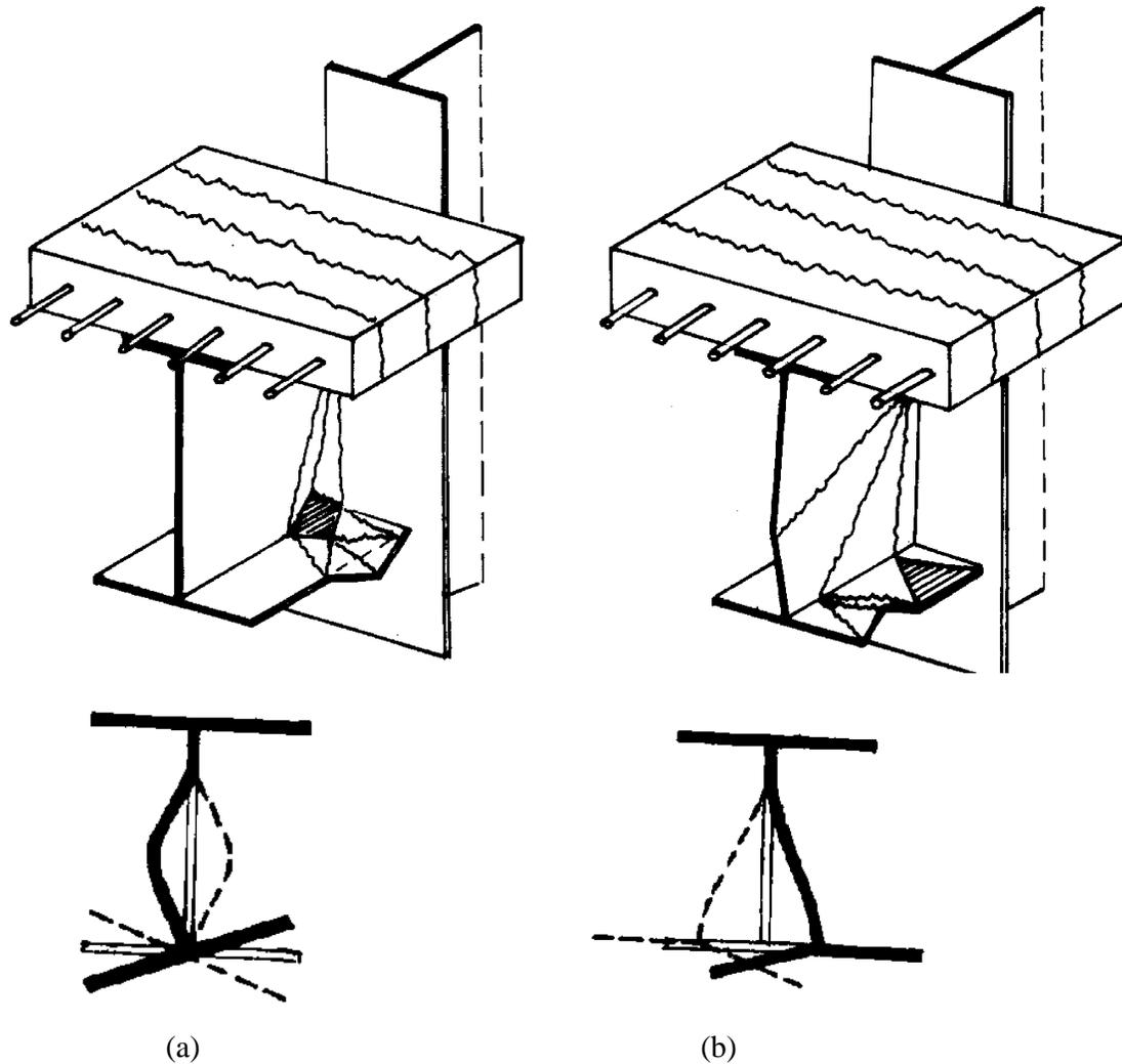
Figure6. Local plastic mechanisms for hogging moments: (a) In-plane mechanism;
