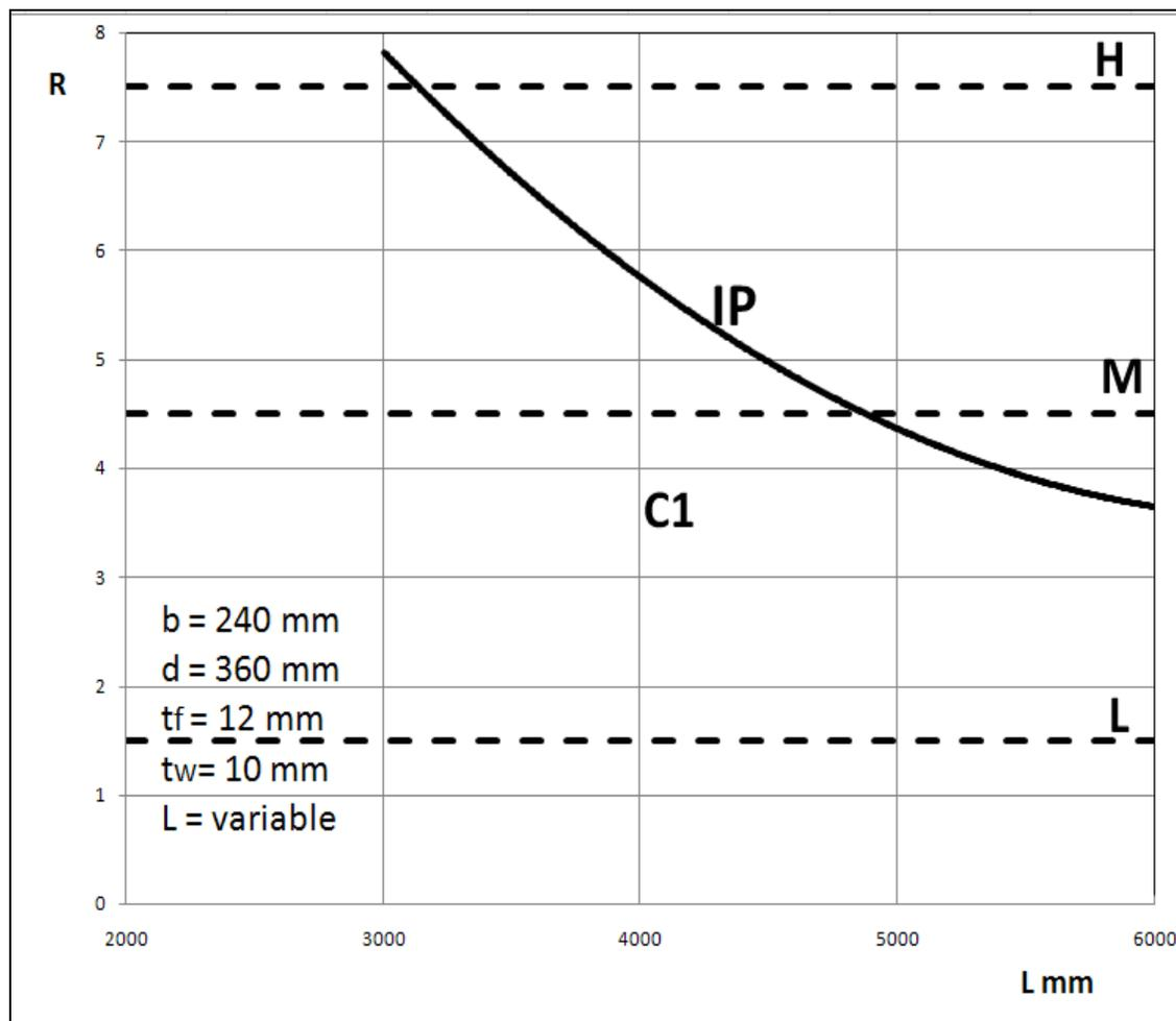
Figure 19. Influence of beam span
