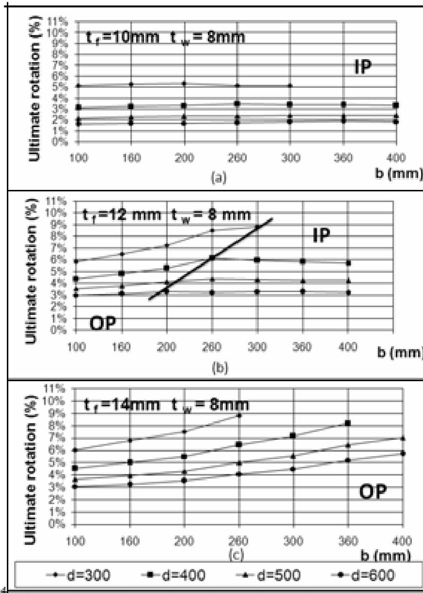
Figure 20. Optimum adjustments for profile dimensions:
