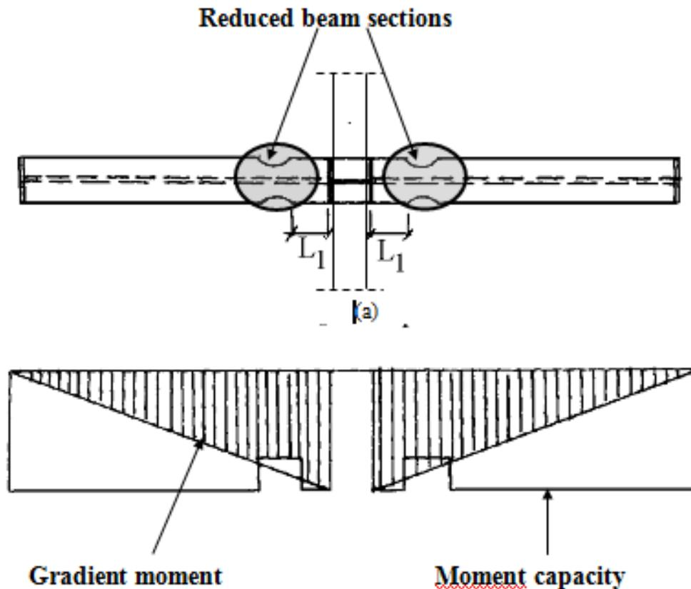
Figure 9. Reduced beam section (RBS): (a) Beam scheme; (b) Positions of RBS
