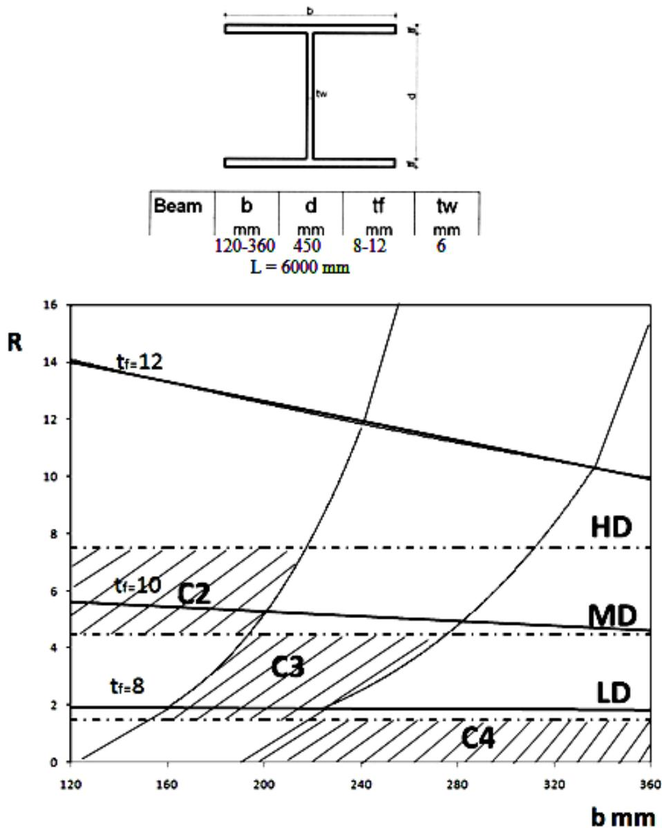
Figure 5. Cross-section versus member classes for a profile with C2 class for web
