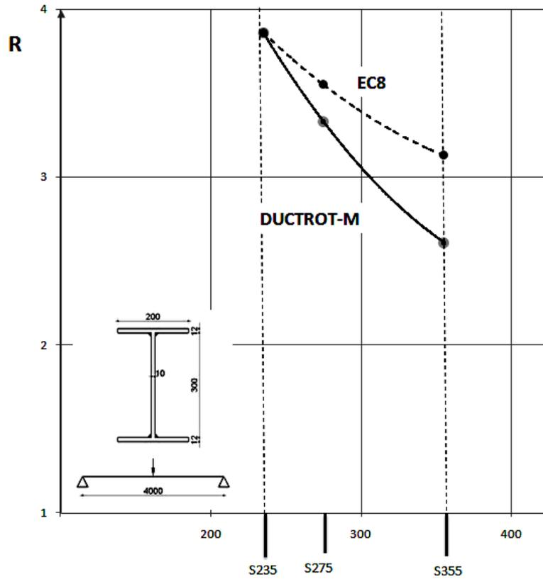
Figure13. Influence of yield stress and steel grade on rotation capacity
