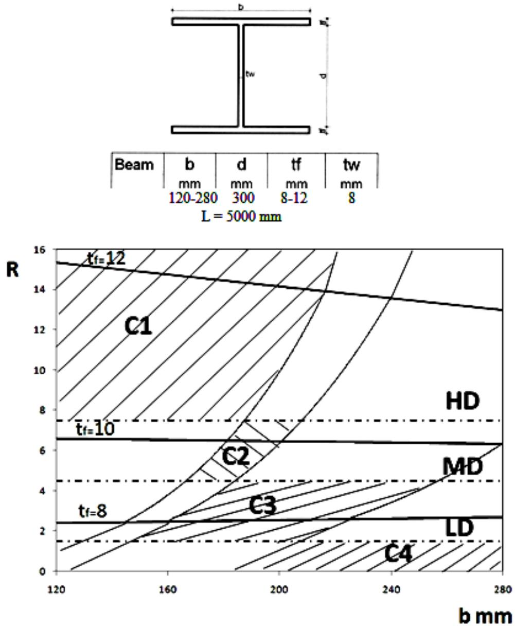
Figure4. Cross-section versus member classes for a profile with C1 class for web
