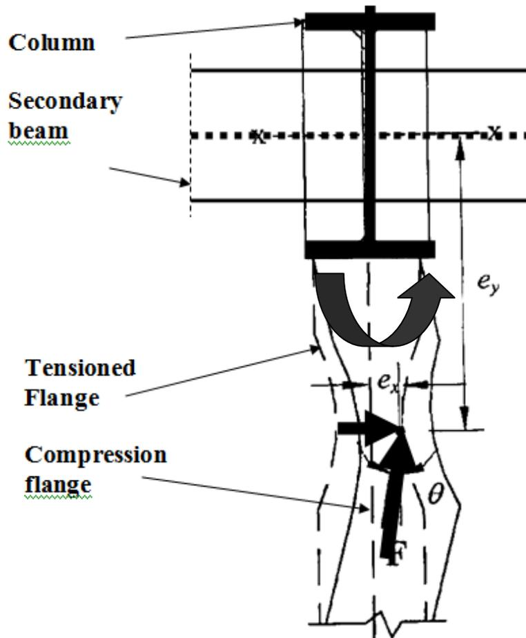
Figure 11. Out-of-plane mechanism for RBS, producing lateral forces
