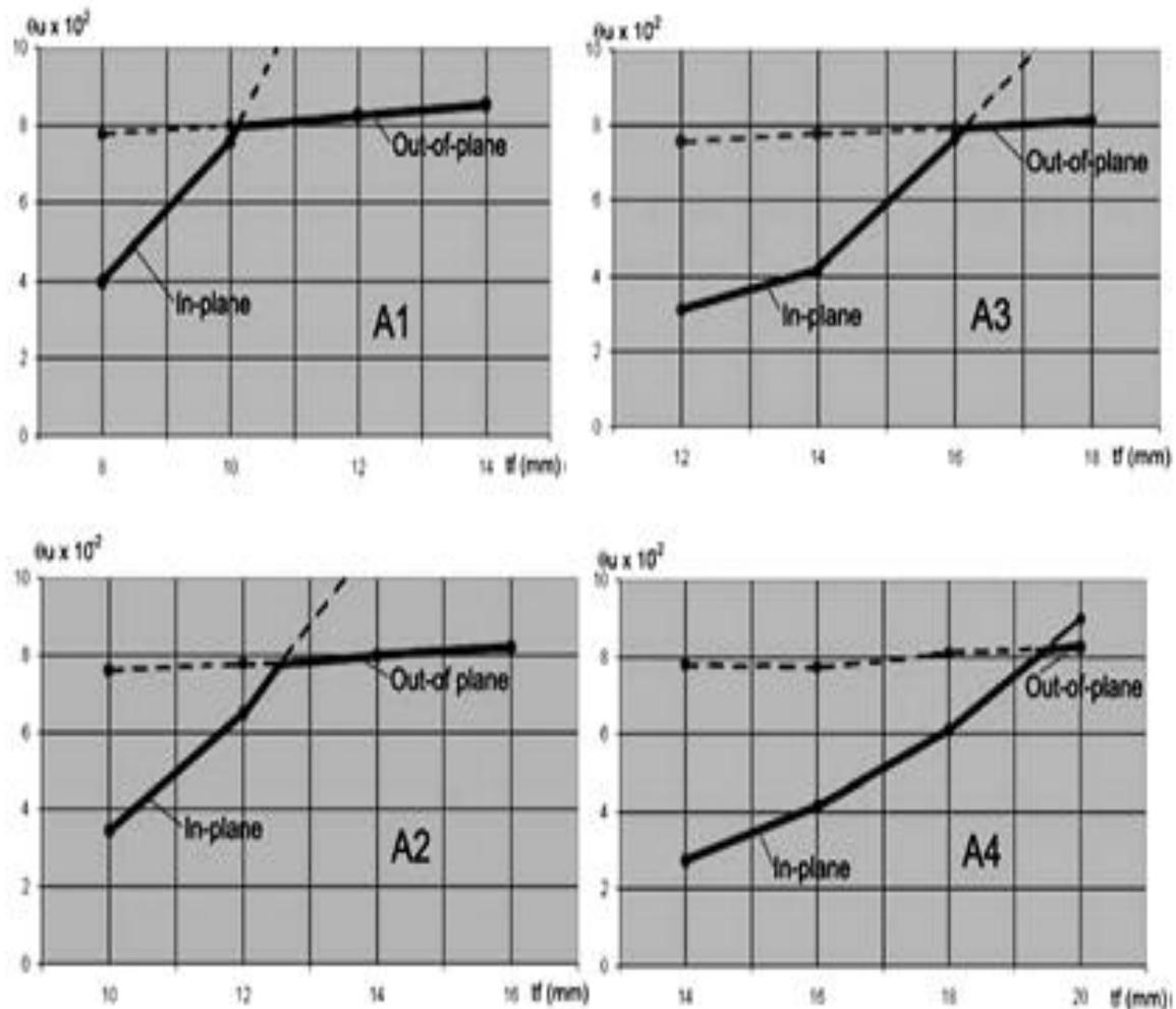
Figure 8. Influence on ultimate rotation of in-plane and out-of-plane mechanisms
