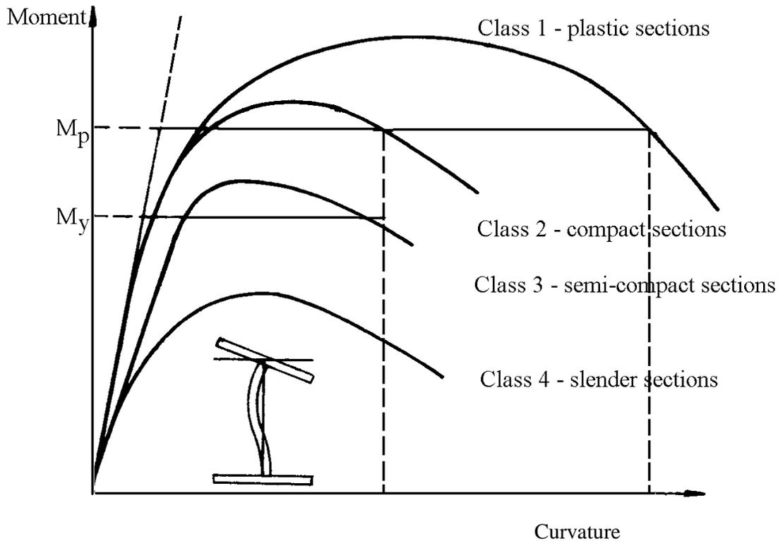
Figure2. Cross-section classes
