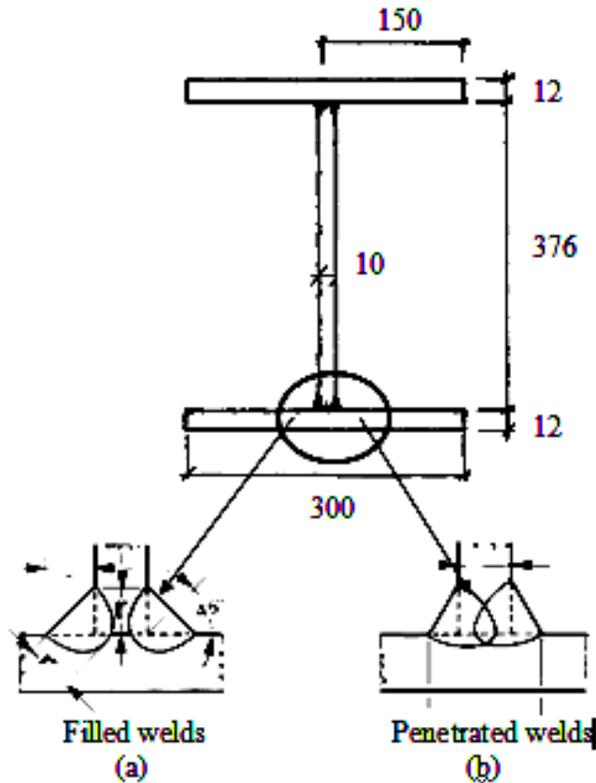
Figure12. Welded profile types: (a) Filled welds; (b) Penetrated welds
