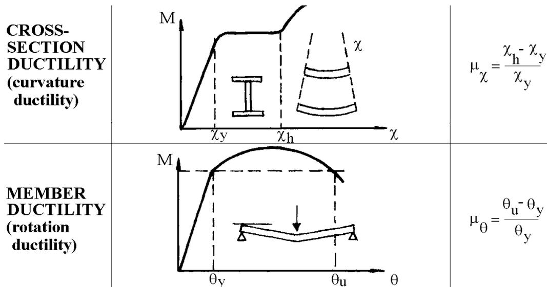
Figure 1. Ductility types: Cross-section and member ductilities
