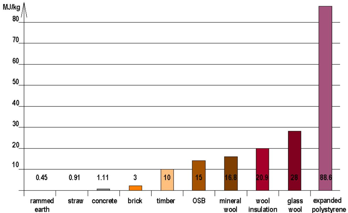
Figure 1. Embodied energy of common building materials
