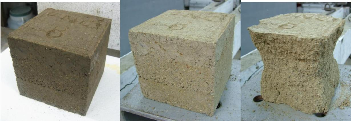
Figure 2. Earth sample after extrusion from the mold, after 28 days of curing and after being tested for compression strength
