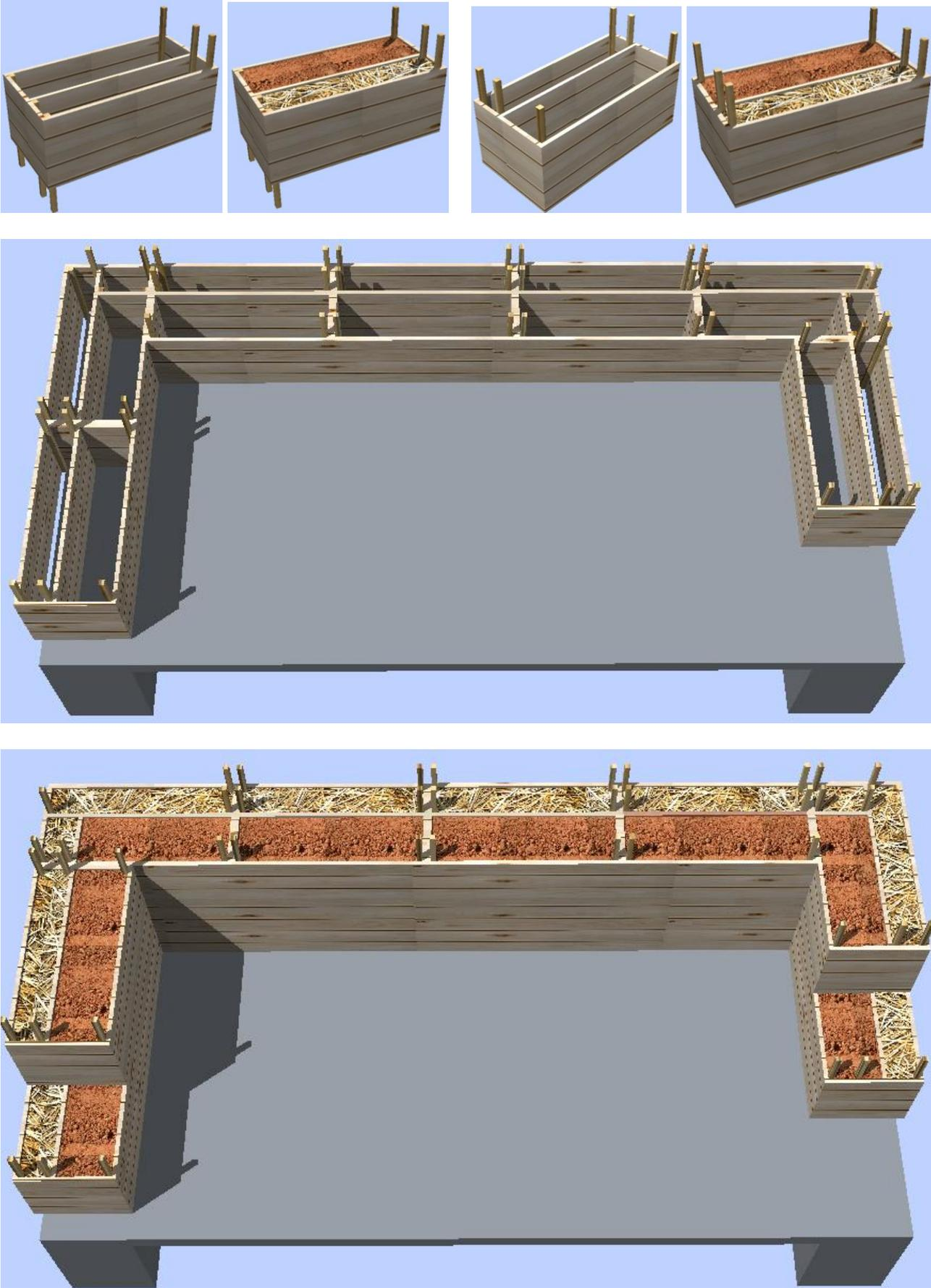
Figure 4. Example of wall built using the box-module
