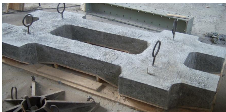
Fig 4. The sleeper after partial de-framing
