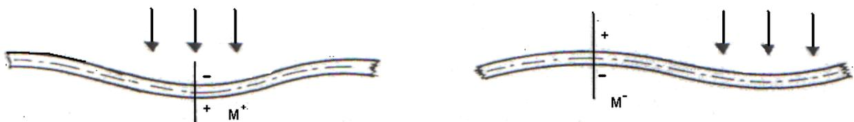
Figure2. Schematic representation of positive and negative bending moments occurred in a section of rail from a passing convoy
