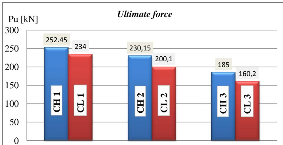
Fig. 4 – Ultimate force for both types of fiber mix studied and for each fiber percentage by volume.
