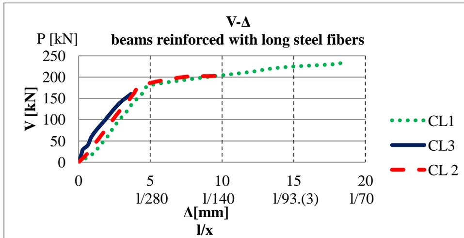
Fig. 5 – Force-deformation diagram for beams reinforced with long steel fibers.
