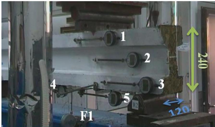
Fig. 3 – testing equipment: 1,2,3 → digital strain gauges; 4,5 → digital strain gauges measuring reinforcement deformation; F1 → deformer for measuring  $\Delta$  deformations.
