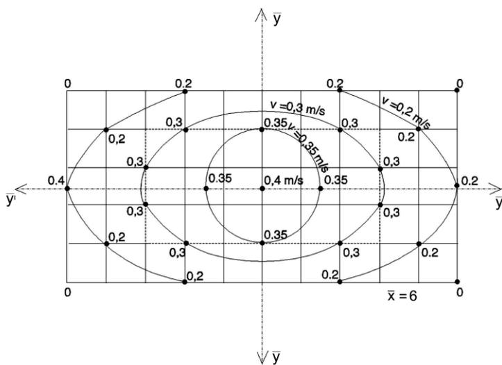
Figure 9. Isokinetic curves for  $\bar{x} = 6$ .
