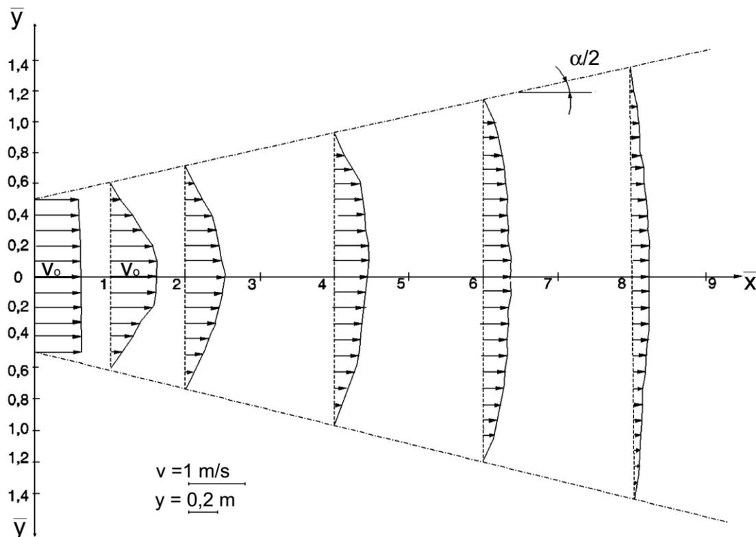
Figure 4. Air velocity hodographs measured in vertical plane.
