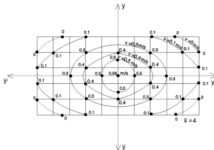
Figure 8. Isokinetic curves for  $\bar{x} = 4$ .
