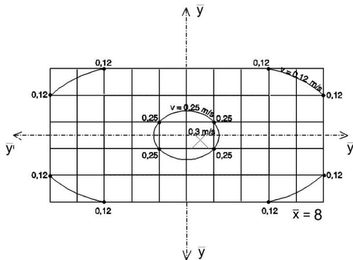
Figure 10. Isokinetic curves for  $\bar{x} = 8$ .
